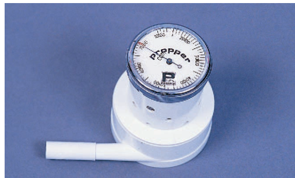
Figure 54.2 A handheld spirometer can be used to measure respiratory air volumes.
