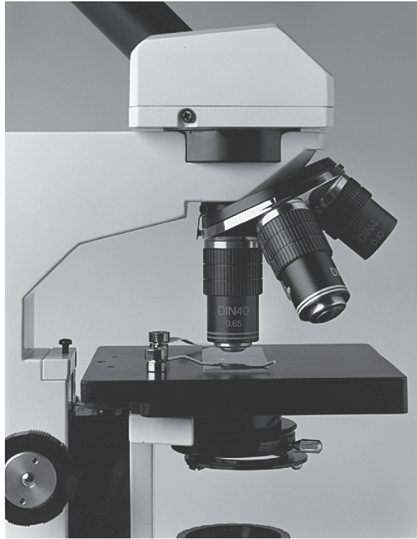
Figure 3.3 When you focus using a particular objective, you can prevent it from touching the specimen by watching from the side.
