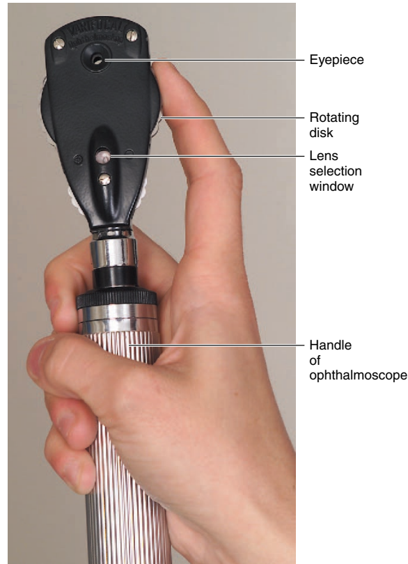
Figure 35.5 The ophthalmoscope is used to examine the interior of the eye.
