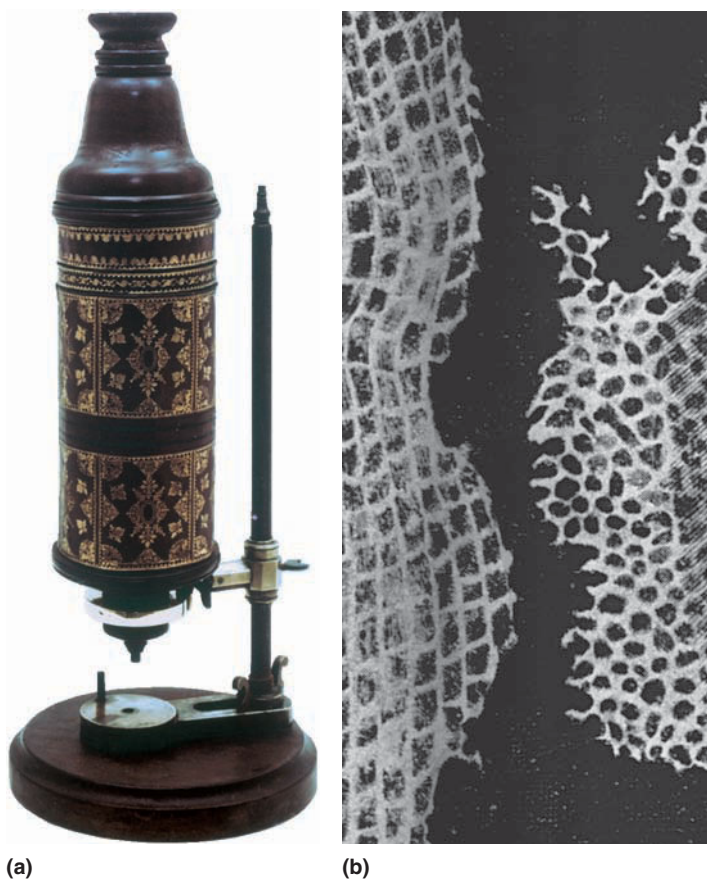
Figure 1.8 Hooke’s Compound Microscope. (a) The compound microscope had a lens at each end of a tubular body. (b) Hooke’s drawing of cork cells, showing the thick cell walls characteristic of plants.
