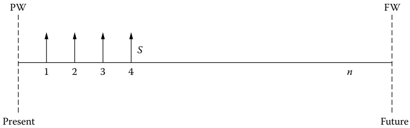
FIGURE 6.2 A uniform series of annual payments and locations of the present and future time frames, shown on the time coordinate axis in terms of number of years n .
