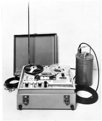
Fig. 3.15 Magnetic-tape recording system (courtesy, R.R. Dibble, 1979), which was used by the author in New Zealand).
