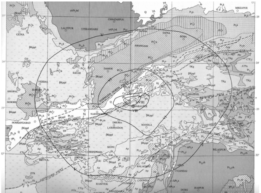
Fig. 7.32 Isoseismal map of the Jabalpur earthquake (GSI, 2000b).
