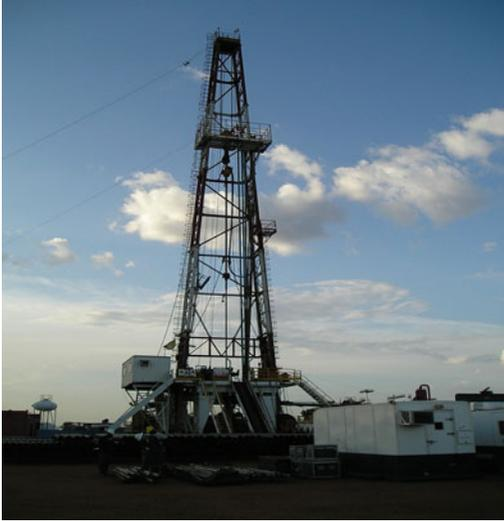
**Fig. 1.8** A typical rotary drilling rig, set up for oil-well drilling operation
