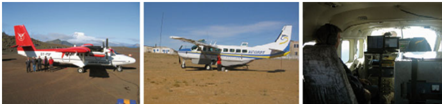
Fig. 3.2 Twin-Otter ( left ) and Cessna Caravan ( center ) are the most popular aircrafts used for airborne gravity today, due to their excellent performance at low air speeds. Right picture shows a typical cabin layout with power conditioner, GPS units, navigation display, and gravimeter in protection box. DTU-Space photos (Jan Mayen Island and Mongolia)
