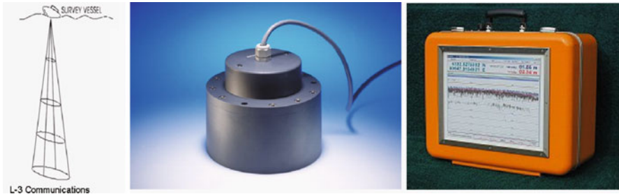
Fig. 8.7 Singlebeam echo sounder ( left ), transducer ( middle , Reson) and record and display unit ( right , Fahrentholtz)
