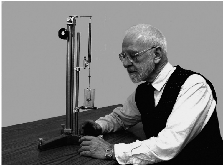
Fig. 2.2 The author using a Jolly balance
