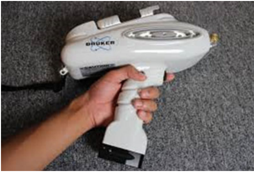
Fig. 8.3 Typical handheld pXRF instrument. Bruker Tracer pXRF model
