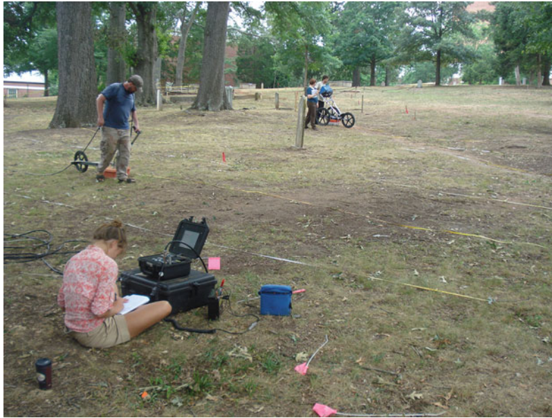
Fig. 5.10 A typical survey grid and GPR units; foreground, a control unit and antenna using a survey wheel; background, another control unit mounted, along with an antenna, on a survey cart. Tapes indicate transect lines (Photograph by the author)
