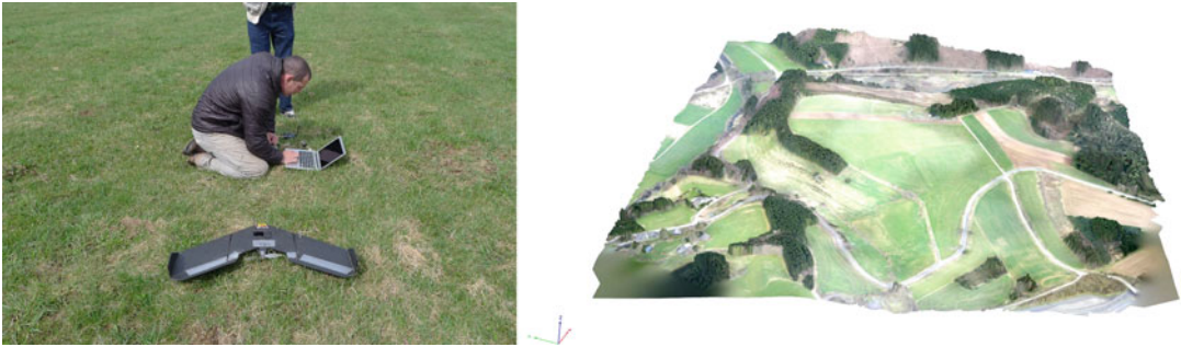
Fig. 2.24 A small, commercial drone (eBee by SenseFly) being preflight programmed for a photographic survey. The photomosaic shown on the right is the result of this particular flight (Photographs courtesy of Chet Walker, shown programming the eBee drone)
