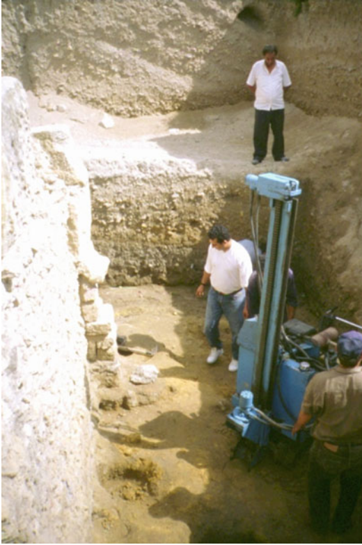
Fig. 4.2 Rotary corer. Shown deployed in the excavation of a Roman era cemetery in urban Tunis, Tunisia, the auger rapidly bores through the clastic sediments. Photograph by Nina Šerman
