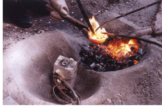
Fig. 9.4 Experimental archaeology. Melting bronze ingots for casting in the stone mold shown in the foreground (Courtesy Latenium, Hauterive, Switzerland)
