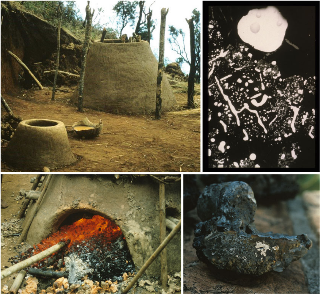
Fig. 9.10 Malawian iron manufacturing, 1982, Chulu, Malawi; above, left, furnaces prior to firing; above, in operation; above, right, micrograph (1000 \times ) showing iron (bright spheres) in bloom matrix; right, bloom
