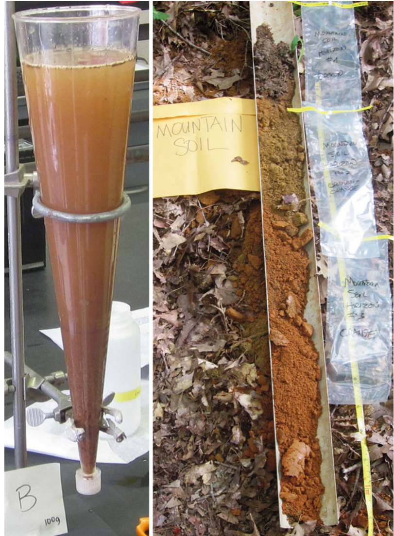
Fig. 4.13 Imhoff cone and soil auger sample. Suspected B horizon shown separating in Imhoff cone
