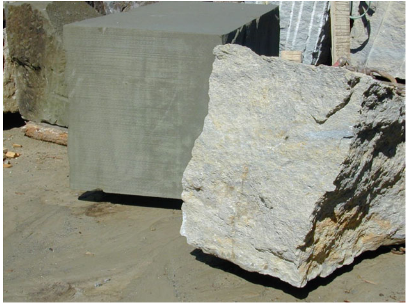
Fig. 6.8 Rear, a siltstone, green “molasse” dimension stone; foreground, a “grès coquille” or bioclastic limestone (Photograph by the author)
