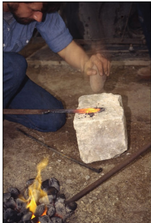
Fig. 9.6 Experimental iron metallurgy. A pit forge, stone hammer, and anvil (Photograph by author)
