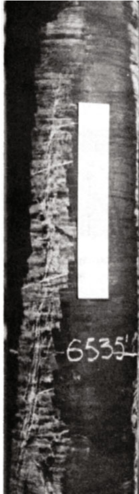
Fig. 3-11. Lynes packer showing impression (enhanced by chalk rubbing) of a vertical joint centered at 6535 ft. Source: Pettitt, 1975c
