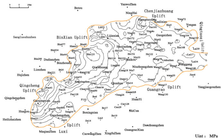
Fig. 4.2 Paleo-pressure map of Es2 member by the end of deposition of the Dongying Formation
