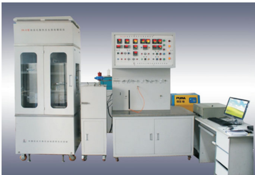
Fig. 2.17 The DK modeling device of hydrocarbon generation and expulsion under in situ conditions
