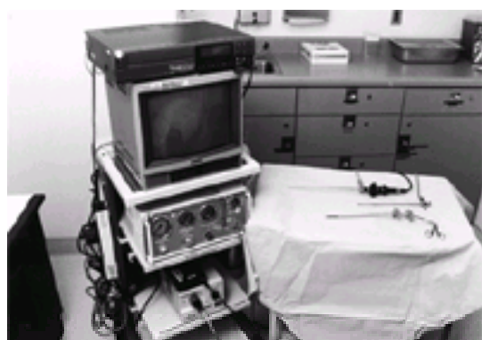
Figure 21.18 Office hysteroscopy equipment. A typical diagnostic hysteroscopy setup. On the table are a hysteroscope, a video camera mount, and diagnostic instruments. On the cart is ( from top ) a super VHS 1/2-inch videotape recorder, a Sony high-resolution monitor, an Olympus hysteroscopic insufflator, and the Olympus video camera base and light source.
