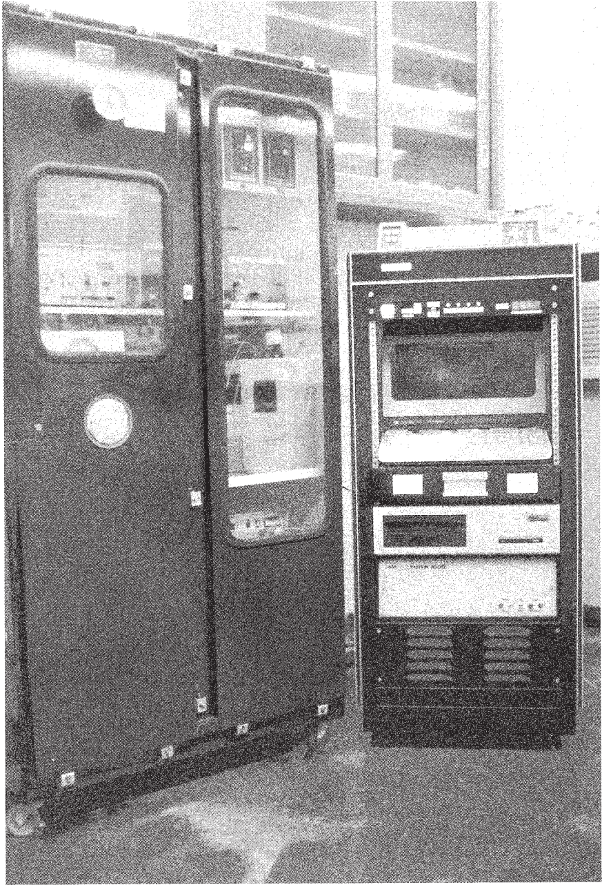
Figure A2.2 Purged enclosure for operation of laboratory HPLC equipment in process area.
