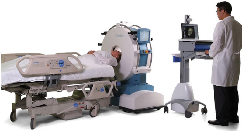
Fig. 9.6 The CereTom is significantly smaller than a traditional scanner, currently with a height of 153 cm, a length of 134 cm, and a width of 73 cm. Its weight is 362 kg. Eight 1.25-mm-wide detectors provide a 10-mm collimated beam. Typical scanning parameters are 120 kV, 7 mA, and a scanning time of 2 seconds. Reconstructed section thicknesses are 1.25 mm in CT-angiography, 5 mm for head scans, and 10 mm for perfusion imaging. Functionally, this machine can be used to perform CT scanning with and without contrast, CT-angiography, CT-perfusion, and CT-fluoroscopy. CereTom Portable CT Scanner. NeuroLogica Website (Available at http://www.neurologica.com/news-media.html )
