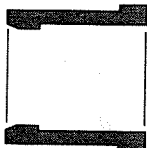
Reducer bushing, spig x slip
