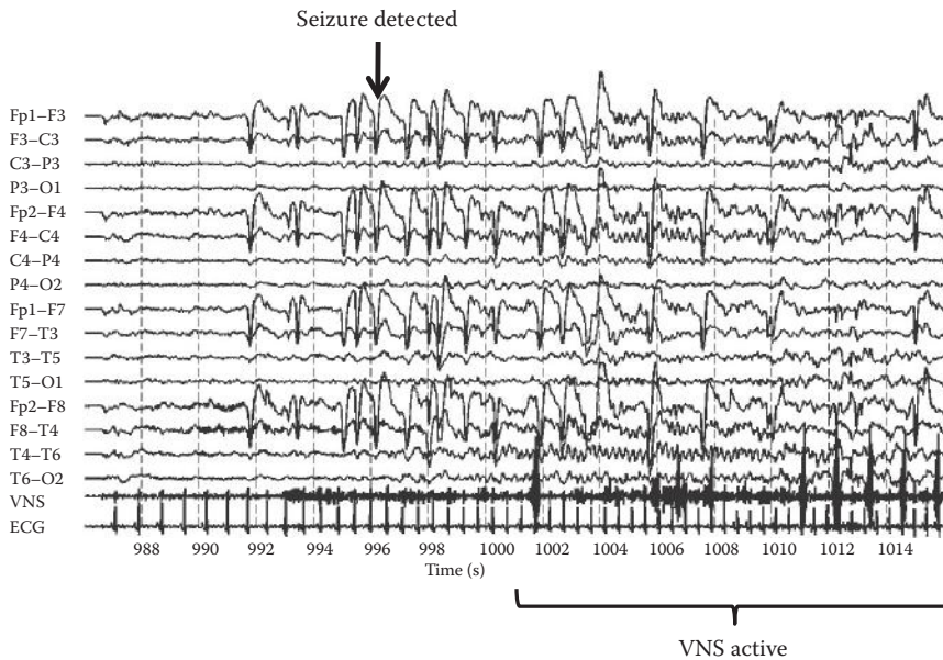
FIGURE 27.5 Seizure detected by computerized system during Patient A's second admission. The seizure, which began at 992 seconds, was detected at 996 seconds and on-demand VNS was initiated in response. The VNS pulse generator became active at 1002 seconds.
