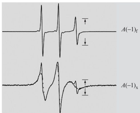
Fig. 21 EPR spectra of spin-labeled CM15 (above) in aqueous solution and (below) in equilibrium with liposomes. The dashed line in the bottom spectra is for peptide 100% membrane bound. Reprinted with permission from Bhargava and Feix (2004). Copyright 2004 by the Biophysical Society.
