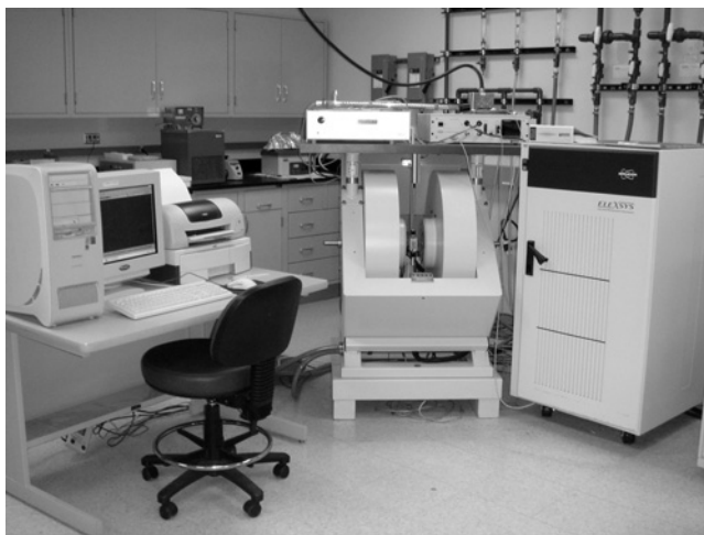
Fig. 2 A typical EPR machine setup with a magnet and microwave source (center), a power supply (right), and a computer for data acquisition (left).
