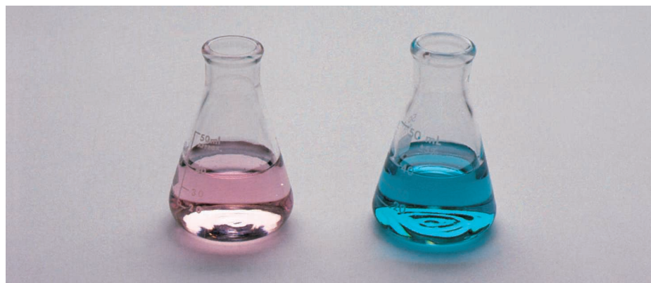
Figure 16.10 (Left) An aqueous cobalt(II) chloride solution. The pink color is due to the presence of \text{Co}(\text{H}_2\text{O})_6^{2+} ions. (Right) After the addition of HCl solution, the solution turns blue because of the formation of the complex \text{CoCl}_4^{2-} ions.
