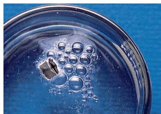
Lithium reacting with water to produce hydrogen gas.
