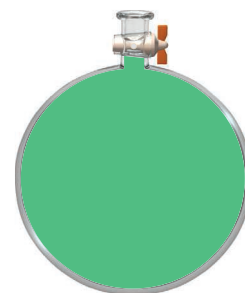
Figure 5.12 An apparatus for measuring the density of a gas. A bulb of known volume is filled with the gas under study at a certain temperature and pressure. First the bulb is weighed, and then it is emptied (evacuated) and weighed again. The difference in masses gives the mass of the gas. Knowing the volume of the bulb, we can calculate the density of the gas. Under atmospheric conditions, 100 mL of air weigh about 0.12 g, an easily measured quantity.
