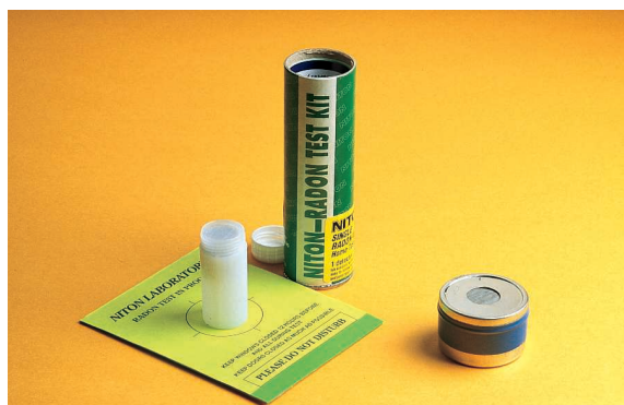
Figure 20.28 Home radon detectors: Long-term track etch (left) and short-term charcoal canister (right).
