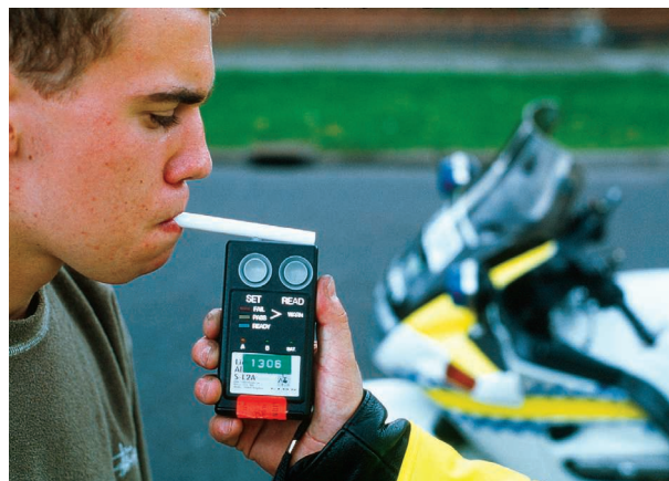
A driver being tested for blood alcohol content with a handheld breathalyzer.
