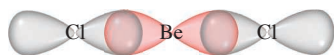
Figure 10.11 The linear geometry of \text{BeCl}_2 can be explained by assuming that \text{Be} is sp -hybridized. The two sp hybrid orbitals overlap with the two chlorine 3p orbitals to form two covalent bonds.
