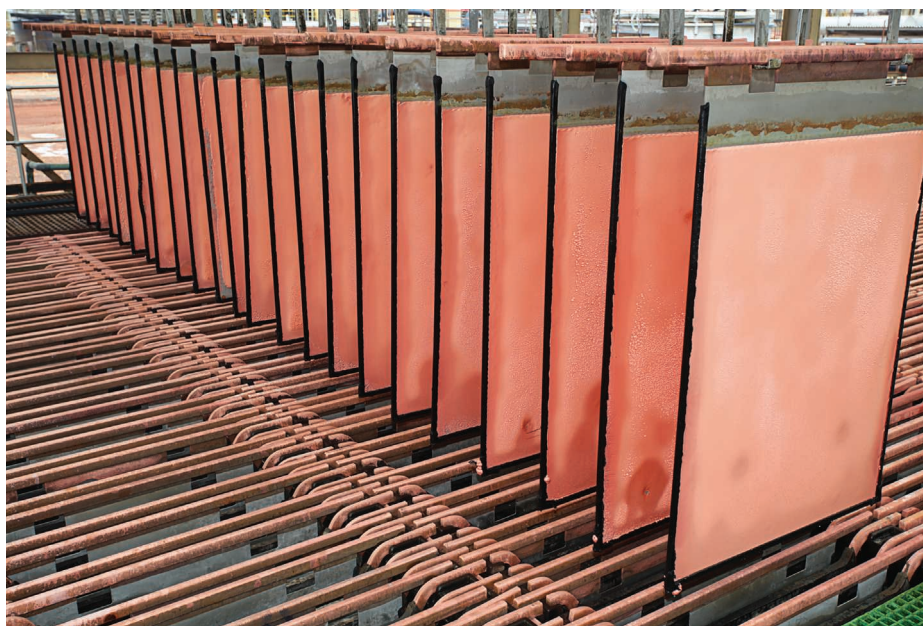
Figure 21.7 Copper cathodes used in the electrorefining process.
