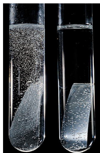
Zn reacts more vigorously with a strong acid like HCl (left) than with a weak acid like CH 3 COOH (right) of the same concentration because there are more H + ions in the former solution.
