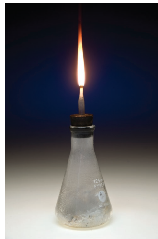
The reaction of calcium carbide ( \text{CaC}_2 ) with water produces acetylene ( \text{C}_2\text{H}_2 ), a flammable gas.
