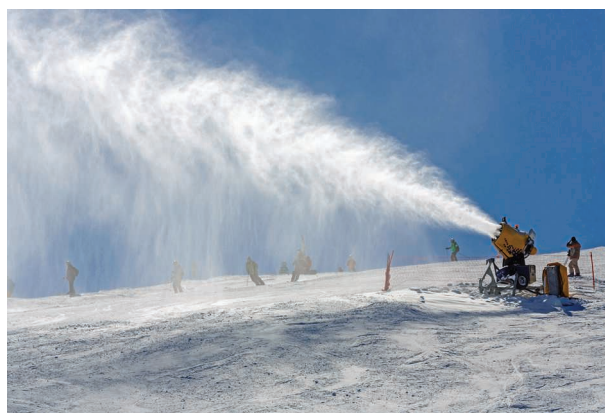
A snowmaking machine in operation.
