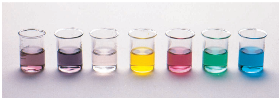
Figure 23.20 Colors of some of the first-row transition metal ions in solution. From left to right: \text{Ti}^{3+} , \text{Cr}^{3+} , \text{Mn}^{2+} , \text{Fe}^{3+} , \text{Co}^{2+} , \text{Ni}^{2+} , \text{Cu}^{2+} . The \text{Sc}^{3+} and \text{V}^{5+} ions are colorless.
