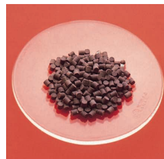
Platinum catalyst on alumina (Al 2 O 3 ) used in hydrogenation.
