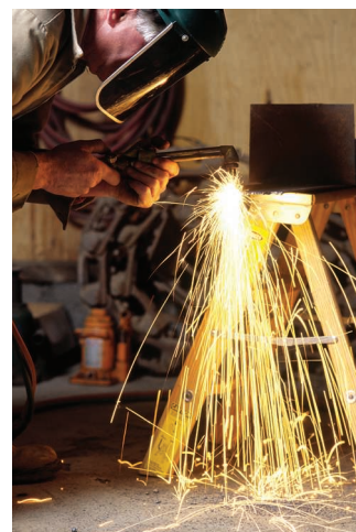
An oxyacetylene torch has a high flame temperature ( 3000^\circ\text{C} ) and is used to weld metals.
