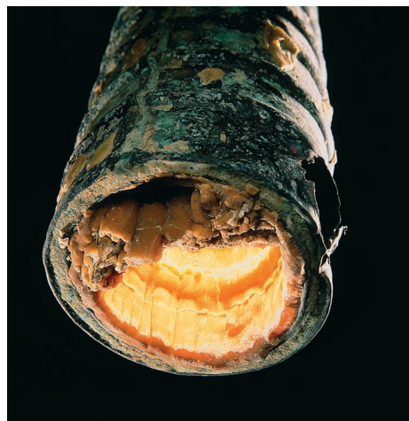
Boiler scale almost fills this hot-water pipe. The deposits consist mostly of \text{CaCO}_3 with some \text{MgCO}_3 .
