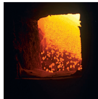
The production of quicklime (CaO) from limestone (CaCO 3 ) in a rotary kiln.
