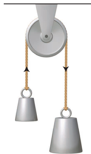
A mechanical analog for coupled reactions. We can make the smaller weight move upward (a nonspontaneous process) by coupling it with the falling of a larger weight.
