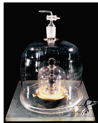
Figure 1.9 The prototype kilogram is made of a platinum-iridium alloy. It is kept in a vault at the International Bureau of Weights and Measures in Sèvres, France. In 2007 it was discovered that the alloy has mysteriously lost about 50 \mu\text{g} !
