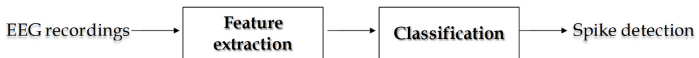
Fig. 2. The spike detection problem seems to be broken down into two main stages: feature extraction and classification. This can be viewed as mapping the N -dimensional EEG pattern space to a F -dimensional feature space (where N \geq F ) and then performing classification in the feature space. In the case of use of raw EEG recordings without feature extraction, this can be seen as the case where the N -dimensional EEG space is mapped onto an identical N -dimensional feature space where classification then takes place (James, 1997).
