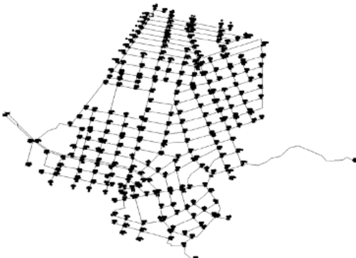
Figure 8.2- Puerto Ayora's network with roof tanks
