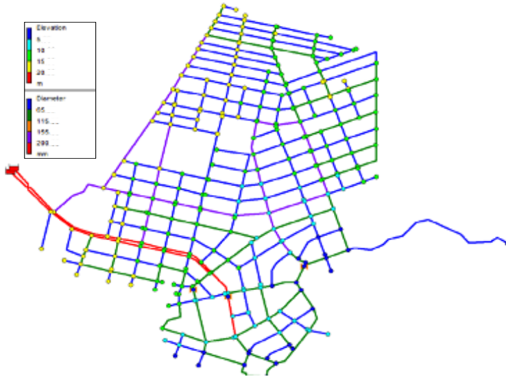
Figure 8.1- Layout of Puerto Ayora water supply network
