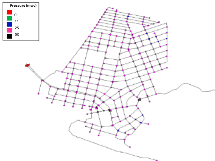
Figure 8.7- Pressures with changing of pipes for a minimum of 25 mwc with moderate growth scenario at year 2045.
