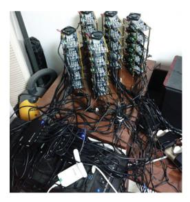
Figure 6.2 Homemade FPGA Mining Rig
