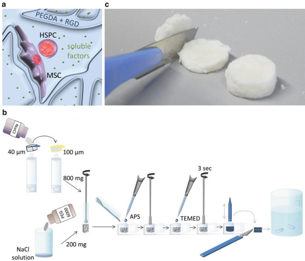
Fig. 1 Overview of macroporous hydrogels and their production. (a) Schematic representation of a macroporous PEGDA hydrogel containing co-polymerized RGD peptide, seeded with HSPCs together with MSCs, and filled with culture medium containing soluble factors. (b) Schematic illustration of the fabrication process of macroporous PEGDA hydrogels. (c) Freshly prepared PEGDA hydrogels ( right ) are cut into two discs using a scalpel ( left )
