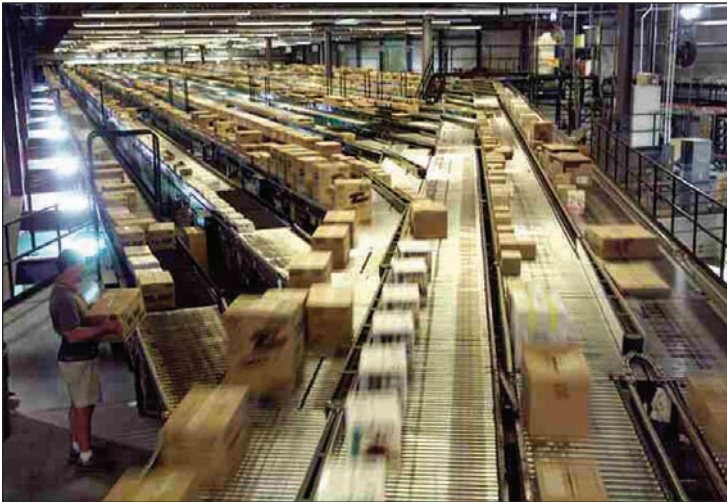
An automated conveyor system moves most cartons to outbound trucks for delivery to stores.
