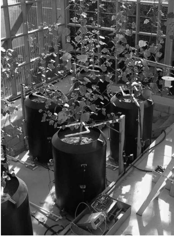
Figure 26.3. Large weighing lysimeters containing 750 L of contaminated sawdust growing one poplar clone, with multiplexed TDR measurements of water content and electrical conductivity. Leachate volume was also monitored continuously, and the chemical concentration assessed regularly. Treatments included varying levels of irrigation and fertilizer application.
