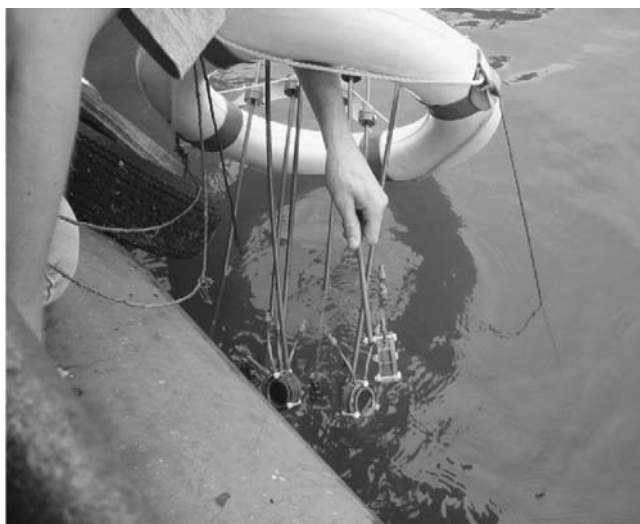
Figure 8.2. In situ measurement field DMT cells.
