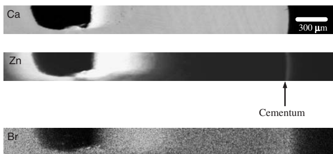
Figure 7.5. X-ray fluorescence maps of a tooth showing top Ca, middle Zn and bottom Br. The Zn enriched cementum region is particularly apparent.
