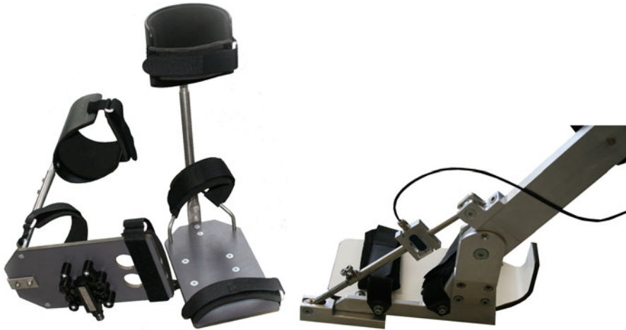
Fig. 11.13 Orthoses for leg stabilization in the parasagittal plane. Left : lightweight orthoses fixing the ankle joint; right : orthosis with a ball bearing and adjustable movement range at the ankle and a force measuring unit for measurements on the generated ankle torque
