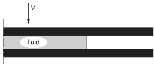
Figure 8.16. Schematic of axisymmetric squeeze flow. Reprinted from Debbaut, J. Non-Newtonian Fluid Mech. , 98 , 15 (2001). Copyright Elsevier.
