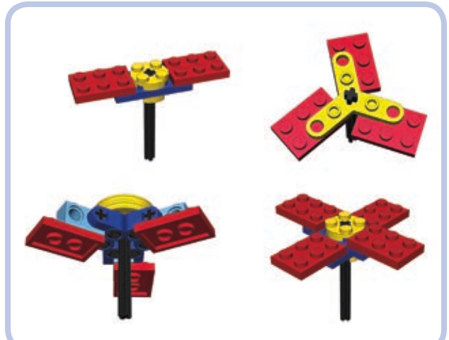
Figure 19-23: Simple hubs with two to four blades
