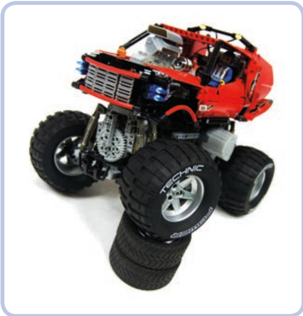
Figure 15-11: My Monster Truck model was a good example of independent suspension. Note that the vertical orientation of both front wheels was identical despite the extreme difference in their heights.
