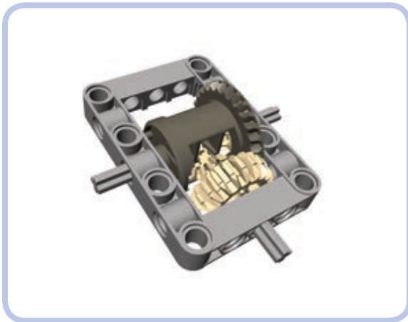
Figure 5-22: A new-type 28-tooth differential gear in a common and robust setup: enclosed inside a 5×7 studless frame and driven by a double-bevel 20-tooth gear
