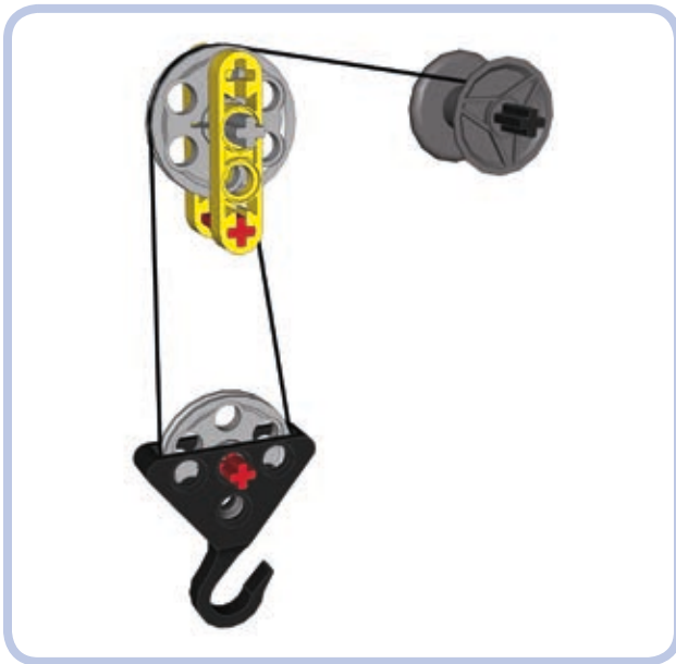
Figure 6-17: This arrangement has two groups, each with a single pulley. The string comes off the upper pulley and around the lower pulley and is then tied to the element that is part of the upper group and remains fixed to it. It's the simplest pulley system, with a mechanical advantage of 2.
