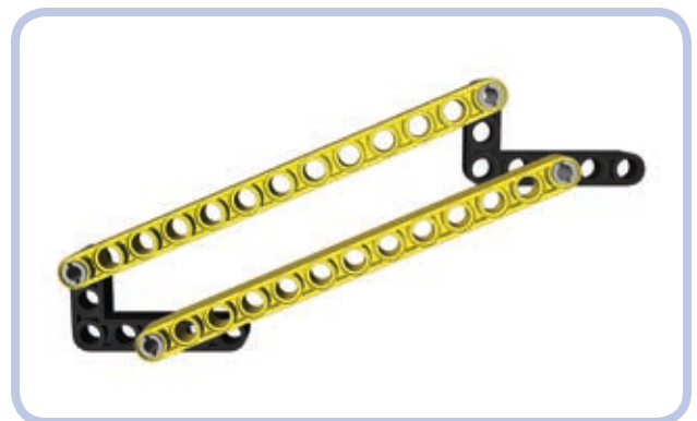
Figure 7-13: The parallel levers are displaced to adjust their range of movement. By moving the upper lever a little backward (left in the figure), we can increase the maximum reach upward at the cost of maximum reach downward.
