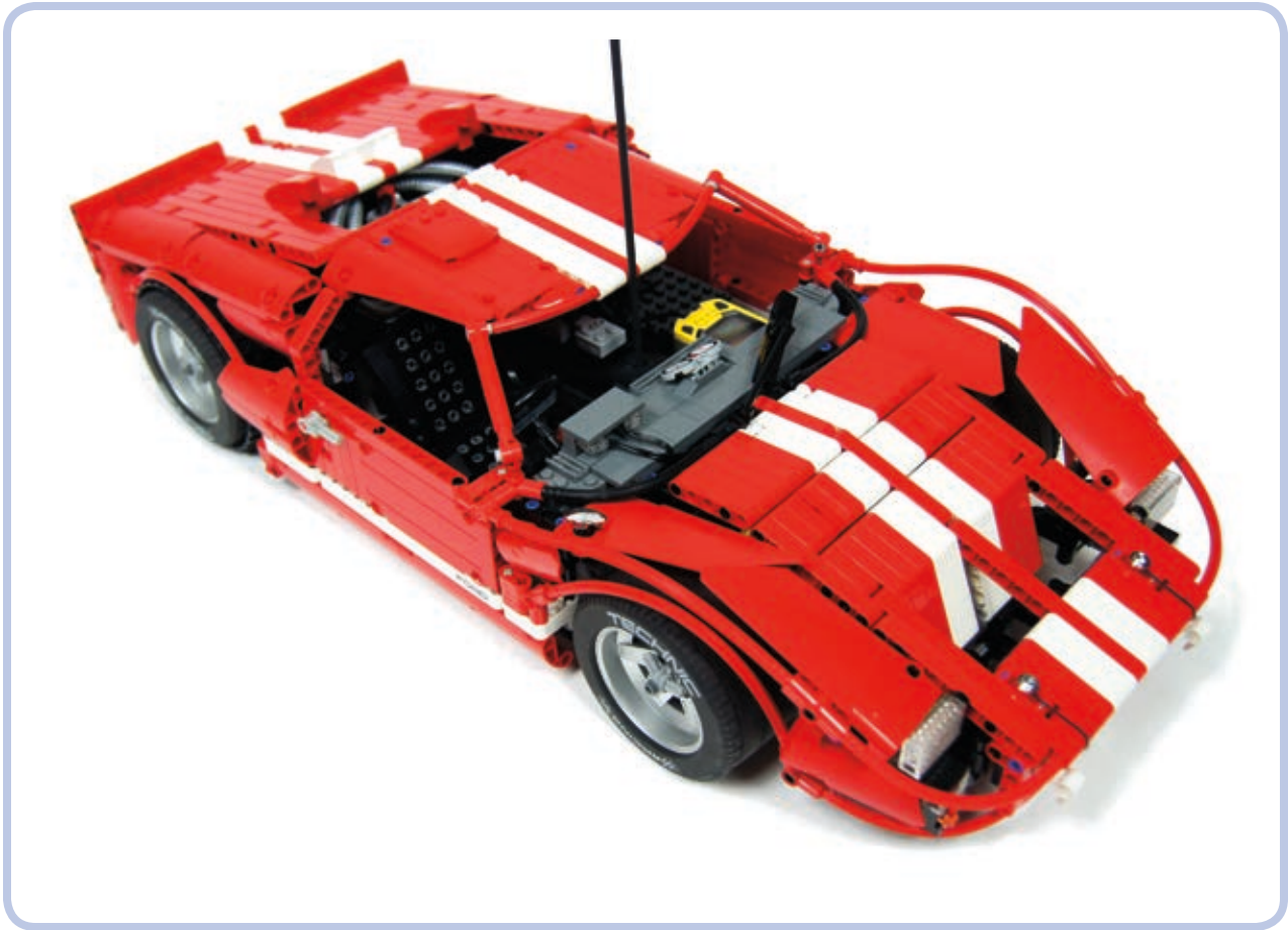
Figure 3-16: My Ford GT40 model had a completely studless body. It combined beams, panels, and flexible axles to re-create the flowing lines of the original car. Studless pieces can create shapes that are impossible to model with bricks, at the cost of certain conventions—in this case, panels approximated the shape of the hood in a way not possible with studfull pieces, but there were gaps between them.
