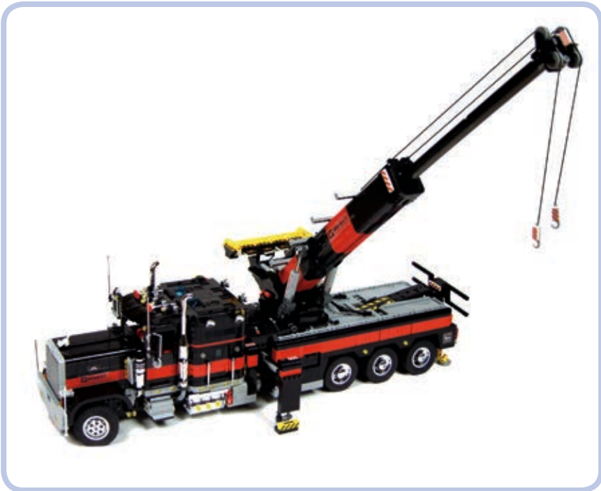
Figure 11-34: My Tow Truck 2 model was very heavy and almost 0.8 m long. It was held together by a massive studfull body frame with two pairs of rails, rigid enough to allow the model to be lifted by hand without any problems. The boom of the truck had its own frame of four studless rails, with the extendable section placed in the middle. It was covered with a studfull shell, which not only made it look better but also improved its rigidity.
