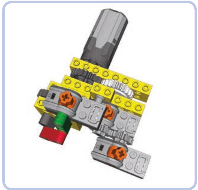
Figure 8-32: A more complex variant uses the Power Functions switch and an eccentric mechanism to make lights flash. The gear is identical to that of the previous figure.
