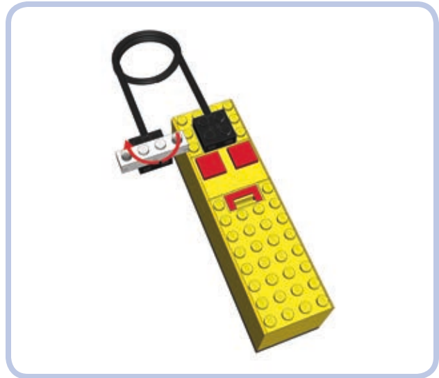
Figure 8-25: A 1x4-stud 9V brick with lights connected to a 9V battery box. By rotating the brick on the plug 180 degrees, we can switch between its lighting modes.
