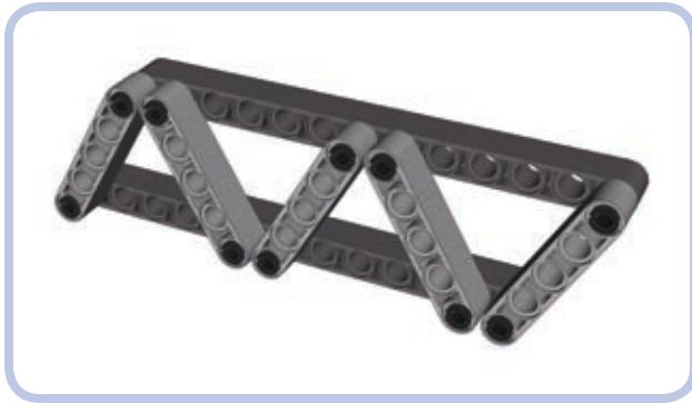
Figure 11-36: A simple truss
