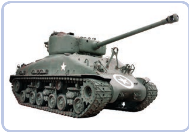
Figure 16-18: The classic Sherman tank used a wheel system that included return rollers.
