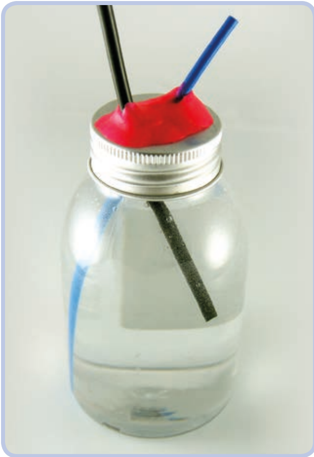
Figure 10-25: A small plastic bottle with a metal cap makes for a very good container. The dark grey elastic hose delivers air, while the blue rigid one lets the water out (note that it can be extended by putting another elastic hose on its end). The cap was punctured in two places to let the hoses through and then sealed with modeling clay (pink).
