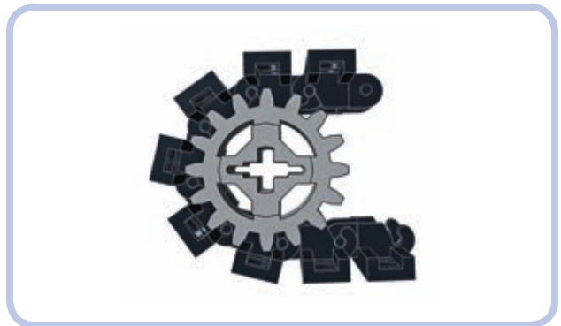
Figure 16-6: A section of older track wrapped around a 16-tooth gear
