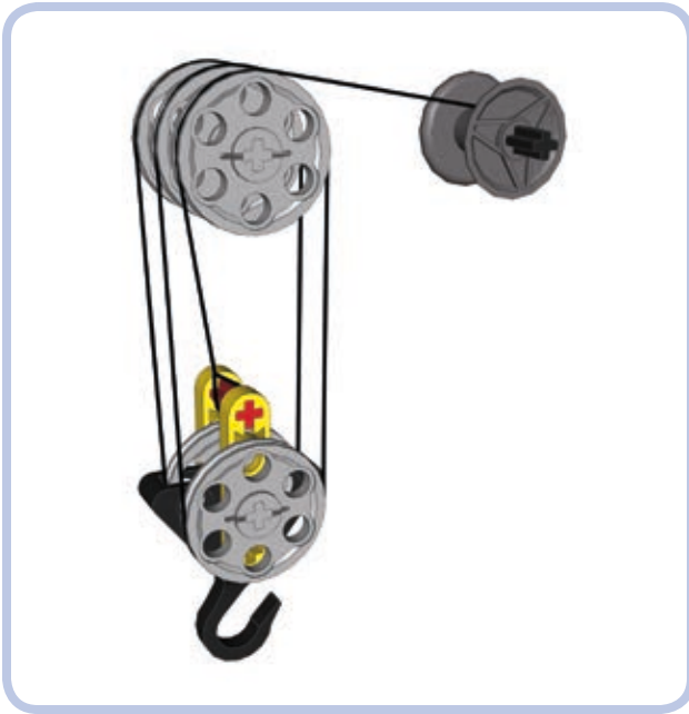
Figure 6-20: This system, called gyn tackle, grants a mechanical advantage of 5.
