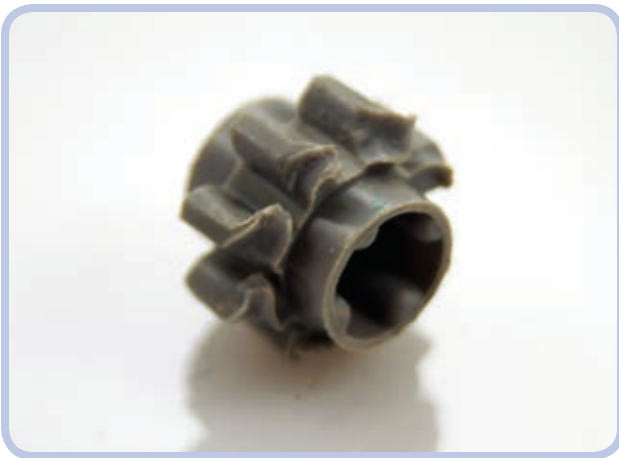
Figure 11-53: This gear's teeth were ground away when it was misaligned to a larger, stronger gear. While the piece itself is new and most of it remains intact, this kind of wear makes the gear unusable.
