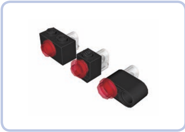
Figure 13-22: The most common examples of installing LEDs in other LEGO pieces. The LEDs fit perfectly into a pin hole. Since their protruding part is less than a stud long, there is still enough room to put in, for example, semitransparent round plates from the other side, creating lights in various colors.
