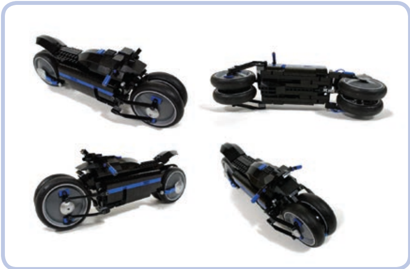
Figure 19-9: The Dodge Tomahawk concept motorcycle comes with double front and rear wheels, thus providing four fulcrums rather than two. I built a motorized model of this bike to prove that it could be motorized and drive stably; however, it couldn't turn because it was too small to house a steering system and a propulsion system at the same time.
