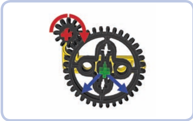
Figure 11-9: The directions of force exerted on the follower gear, which is located below and to the side of the driver gear
