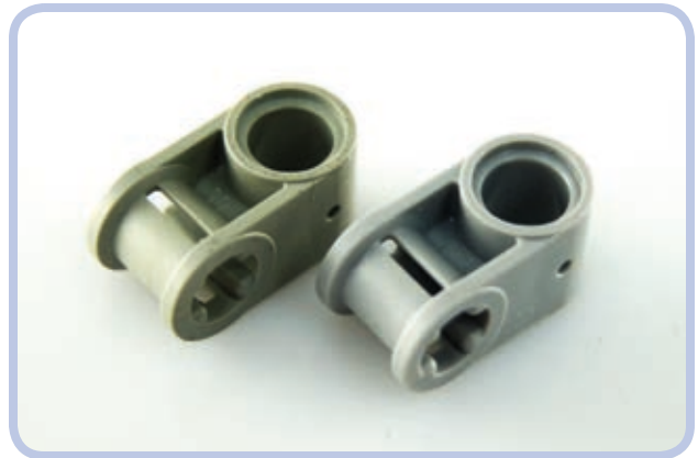
Figure 11-50: A connector: old (left) and new (right). Even though the old piece is free from damage or visible wear, the difference is obvious.
