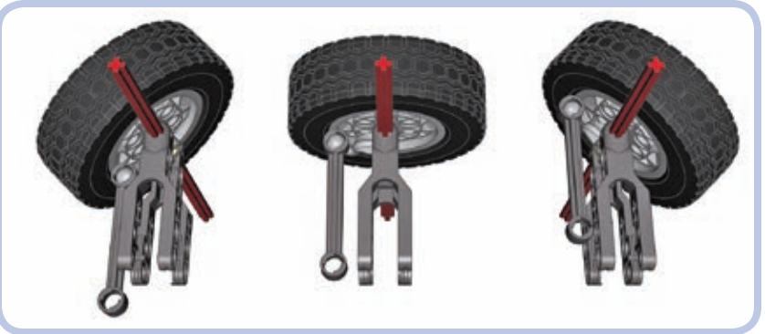
Figure 21-11: When steered, a typical LEGO wheel rotates around a pivot point that is often well outside it. It requires more free space around the wheel, and it also makes the front of the vehicle move while steering in place.
