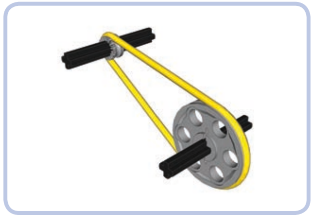
Figure 4-8: A half bush and a wedge belt wheel both have grooves for LEGO rubber bands and can be used as pulleys.
