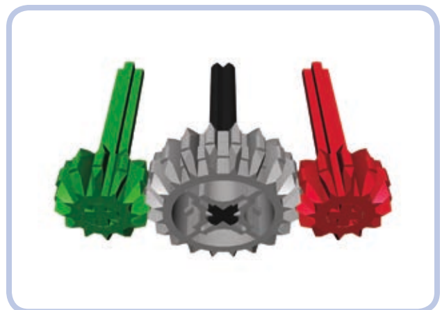
Figure 5-5: Three gears meshed one by one, with the idler gear in grey. The idler's axle serves only as its mounting point.
