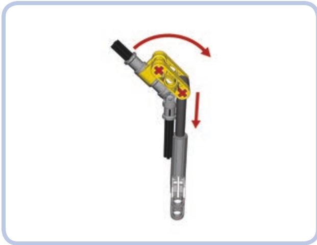
Figure 19-21: An example of a simple rotor-tilting mechanism. The black axles with a universal joint are the driveshaft, connecting the rotor on the top with a motor on the bottom. Retracting and extending the linear actuator changes the angle of the axle above the joint and thus of the whole rotor.
