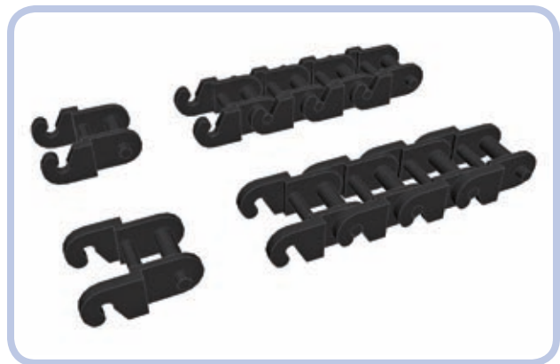
Figure 6-2: A single chain link and a section of four connected links, shown with slots facing upward and downward. In theory, the chain is less likely to come apart when its slots face the gear, but in practice, the difference is negligible.
