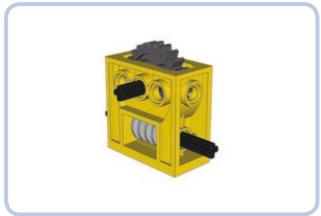
Figure 11-27: The LEGO casing for the worm gear is very sturdy and quite common, but it works only with a 24-tooth follower gear. It's also better suited for studfull structures than for studless ones.
