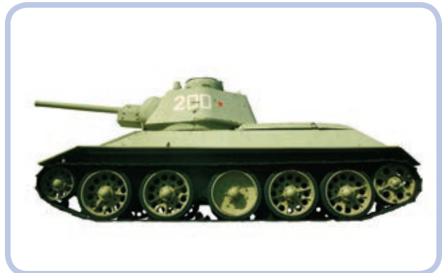
Figure 16-17: Soviet tanks from the World War II era—such as this T34—used road wheels so big that they had contact with both the lower and upper portion of the track, thus eliminating the need for return rollers.
