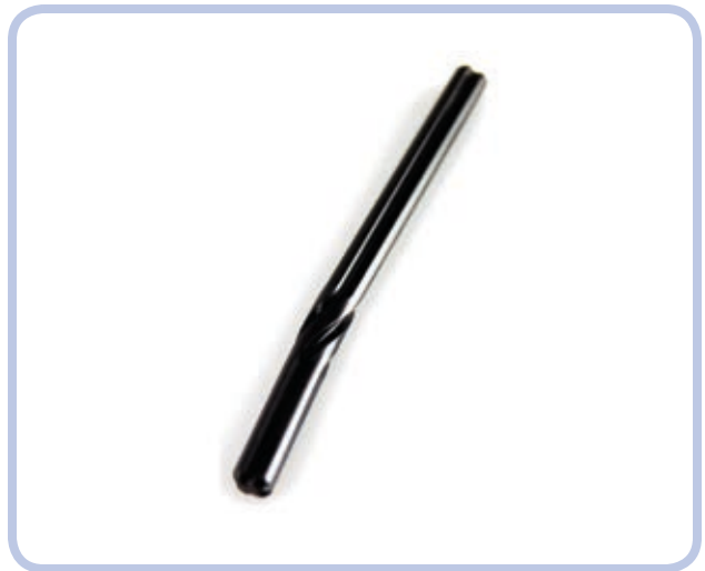
Figure 11-17: Axles are much more elastic than they might seem. This one has been twisted permanently by a PF XL motor.
