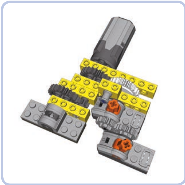
Figure 8-31: Two hard-coupled switches connected to a motorized flashing-light mechanism that uses an old 9V switch. Note the gear down between the motor and the 9V switch—it lowers the flashing rate of the lights to a realistic value.
