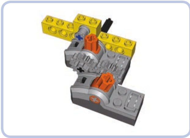
Figure 8-30: Two hard-coupled switches with one of them blocked. The hard-coupling makes the block work on both switches.
