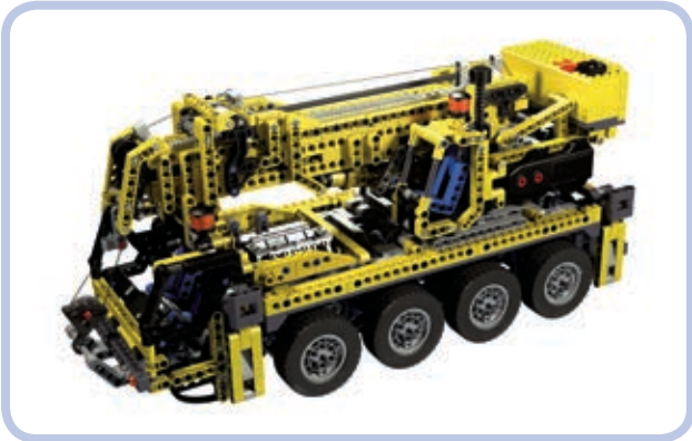
Figure 3-22: The acclaimed 8421 Mobile Crane set is primarily studless, but it uses a combination of bricks and plates for the most heavily loaded part of the boom.
