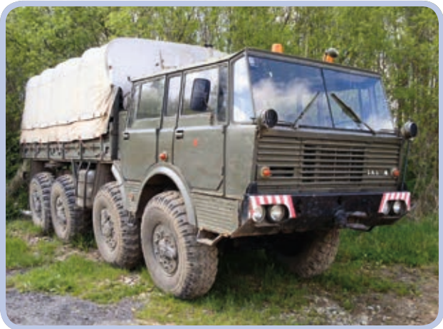
Figure 15-13: The default position of the Tatra-type suspension offers extra ground clearance. This “bowed” look can be mistaken for damage or warping.
