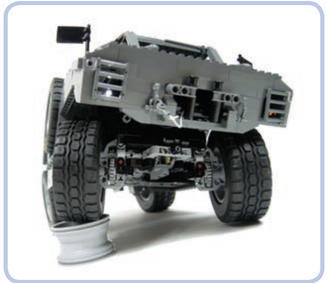
Figure 15-22: My model of the RG-35 4x4 MRAP vehicle made use of LEGO hubs to achieve an impressive ground clearance exceeding 6 studs.
