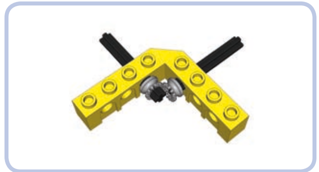
Figure 4-12: Toothed half bushes working as bevel gears. Note the quarter-stud spacings between the half bushes and the adjacent brick. Meshed this way, the half bushes can actually work very smoothly, provided high torque is not applied.
