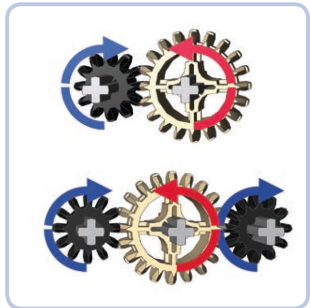
Figure 5-9: An even number of meshed gears (left) and an odd number of meshed gears (right)
