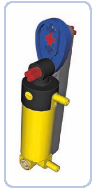
Figure 10-16: To make the cylinder extend fully, we need its tip to be mounted 1.5 studs away from the shaft. A piece called a Technic cam allows this.
