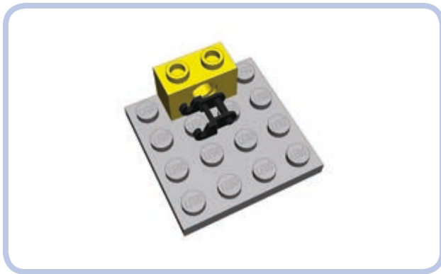
Figure 6-3: An individual chain link is very small and practically impossible to combine with any other type of LEGO piece.
