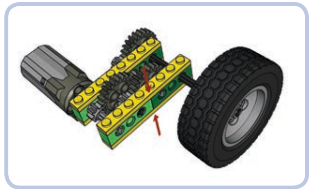
Figure 11-3: The critical connection in the mechanism from Figure 13-2 is marked by a red arrow here. This connection lies between two separate bricks and is held together merely by the clutching force of two 1×8 plates (yellow); therefore, it can be broken easily.
