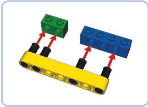
Figure 3-32: Beams can be easily connected with bricks using pins. Note that we can choose regular Technic bricks (blue) or bricks with centered pin holes (green) to adjust the alignment.
