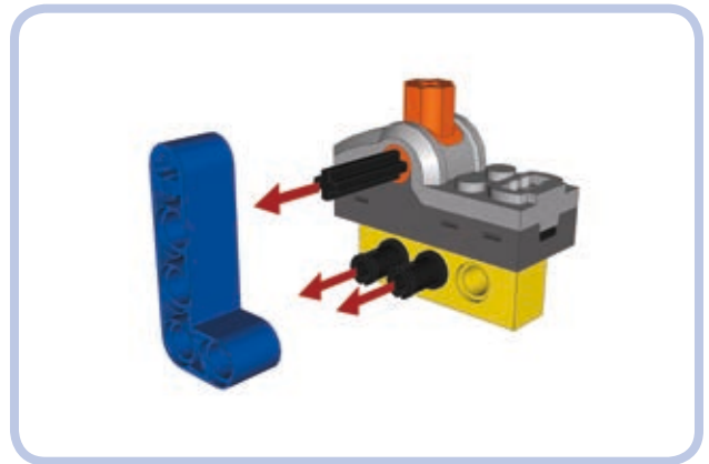
Figure 3-38: The Power Functions switch is easily connected to studfull pieces, but creating a rigid connection with a studless piece is more challenging.
