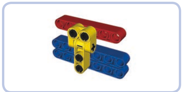
Figure 3-43: A combination of two connectors (yellow) used to align a 6-stud-long piece (red) to the center of a 7-stud-long structure (blue)
