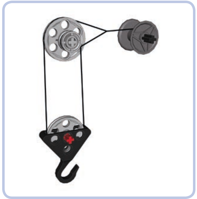
Figure 6-22: Differential block and tackle with two independent pulleys of different diameters in the upper block
