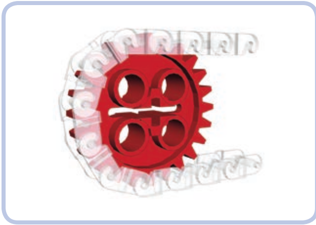
Figure 6-7: A close-up view of the chain wrapped around a gear shows that each link occupies two teeth. The section of the chain that has contact with the gear has no play in it, and its elasticity is minimized.
