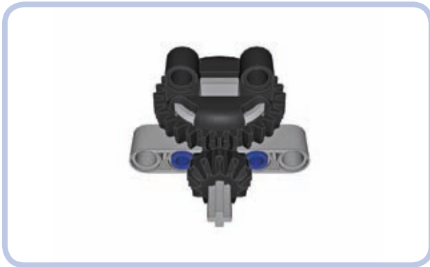
Figure 5-24: A small turntable meshed with a double-bevel 12-tooth gear
