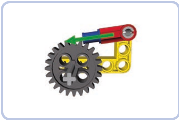
Figure 8-8: The angle of the pawl should be such that the line coming out of its mounting point aims slightly below the gear's rim.
