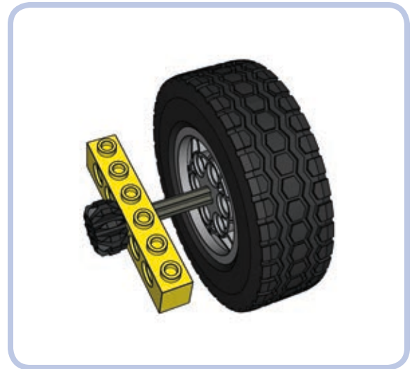
Figure 4-4: Using the 5.5L axle with stop
