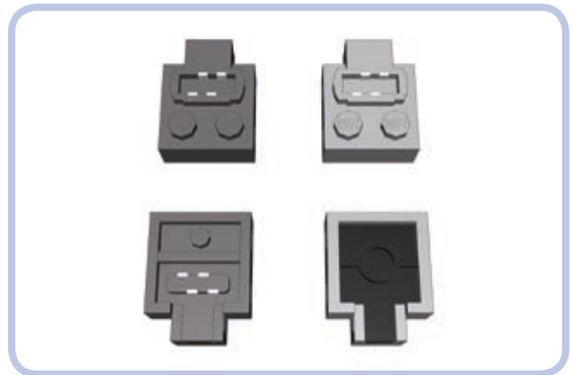
Figure 13-18: Top and bottom view of a regular Power Functions plug (left) and the adapter plug (right). Each extension wire comes with one plug of each type.
