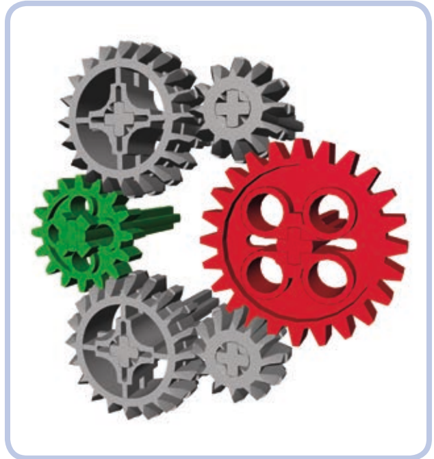
Figure 5-8: All the middle gears in this picture are idler gears. They do not affect how torque and speed are transformed between the driver gear and the follower gear.
