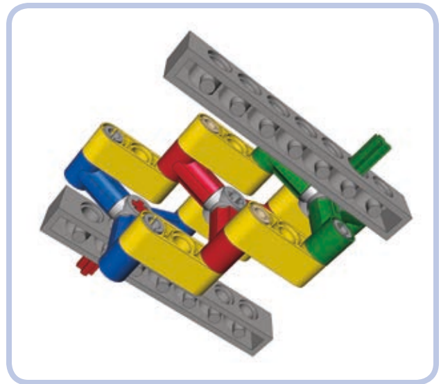
Figure 8-19: A Schmidt coupling with three triangles (in green, red, and blue) and six links (yellow). Note that the middle triangle (red) doesn't need any support—it can even move as the coupling works.
