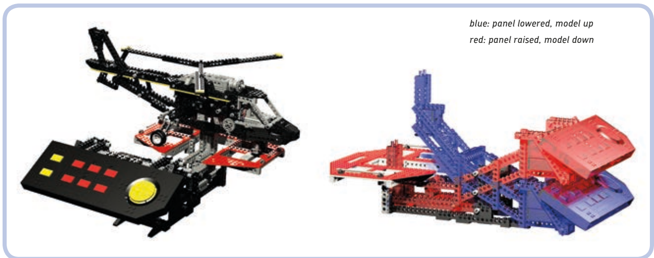
Figure 19-14: The LEGO 8485 Control Center II set features a large helicopter on a simple boom (left). By manually lowering the control panel (right), which acts as the helicopter's counterbalance on the boom, we can lift the model up and simulate the movement of free flight—for example, the tilting of the hull.
