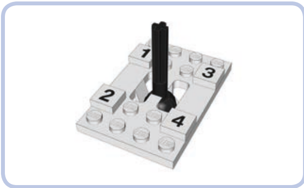
Figure 17-2: The unique shift stick from the 8880 set, the first LEGO set with a nonlinear and synchronized transmission. The transmission has 4 speeds, and the stick can move in an H pattern, allowing it to shift from one gear to any other.
