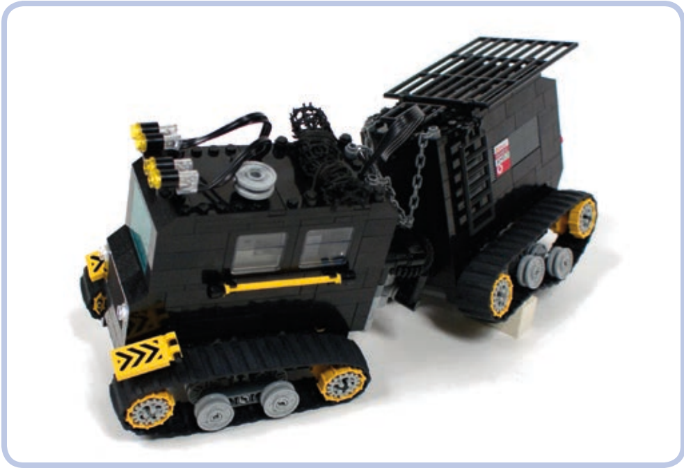
Figure 19-10: The Swedish Haggglunds BV 206 personnel carrier consisted of two parts connected by an articulated joint. This very tiny model housed one steering and two propulsion motors, a battery and an IR receiver, while its simple suspension was located entirely within the tracks.
