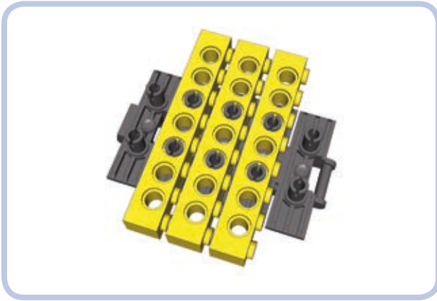
Figure 16-11: Section of the newer track with bricks attached
