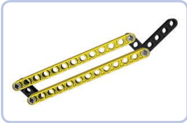
Figure 7-14: The functioning of the parallel levers relies on the positions of their points of attachment. These positions can be made identical on both ends using various elements set at various angles.
