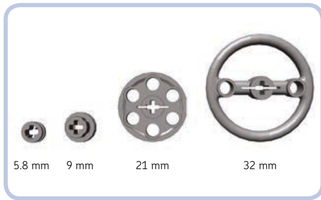
Figure 6-10: The diameters of the pulleys, which determine their ratios
