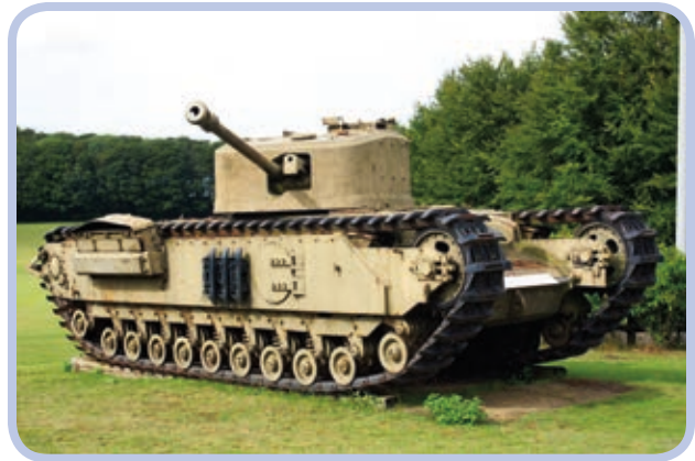
Figure 16-15: With 11 road wheels per track, the British Churchill tank is an extreme example of using a design that includes many small road wheels.
