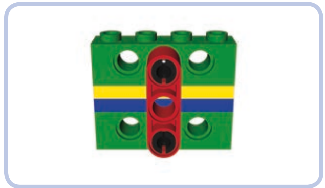
Figure 2-16: The basic rule of alignment for studless and studded pieces: Holes in two bricks separated by two plates are exactly 3 studs apart.
