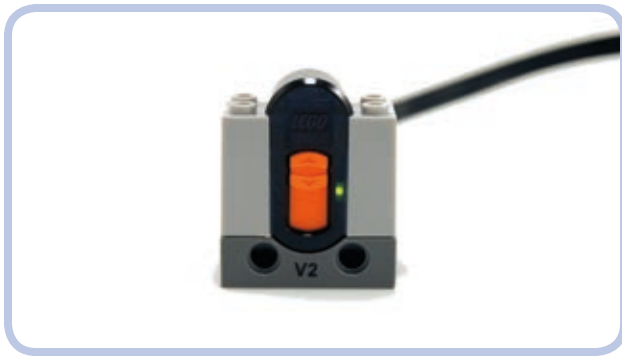
Figure 13-9: The V2 Power Functions receiver. Note the shining indicator LED.
