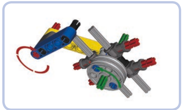
Figure 8-21: A simple Geneva mechanism with an input (red) and an output (green). Each rotation of the input advances the output by a quarter rotation—that is, 90 degrees.
