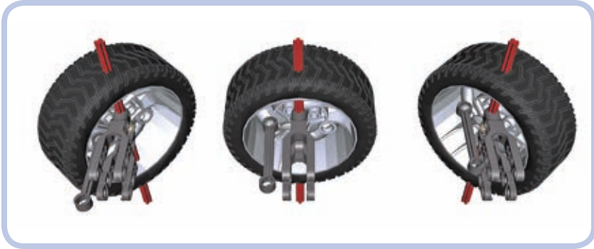
Figure 21-10: Of all existing LEGO wheels, only the 8448 set's wheels rotate around their centers when steered—and they are still a little off.
