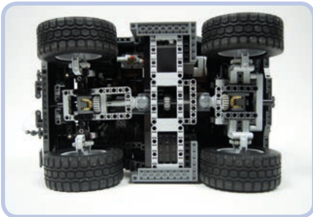
Figure 3-29: My model of the RG-35 4×4 MRAP vehicle (an armored personnel carrier) combined a completely studless chassis with a fully studfull body. The realistic model was extremely compact, but its densely built body made it top-heavy.
