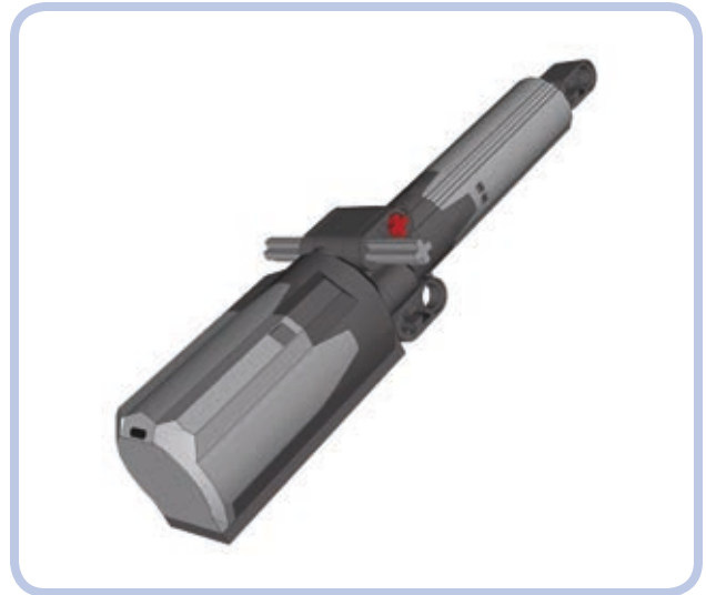
Figure 13-13: The bracket with fixed mounting can connect a motor and actuator as a single unit that can pivot around one of the mounting axles (light grey).
