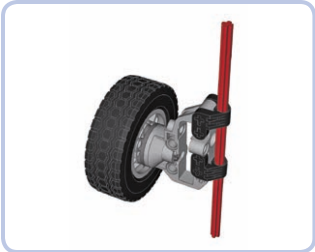
Figure 21-12: LEGO portal axles are worst in terms of steering geometry. Their pivot point is located between the chassis and the gear hub, quite far from the actual wheel.
