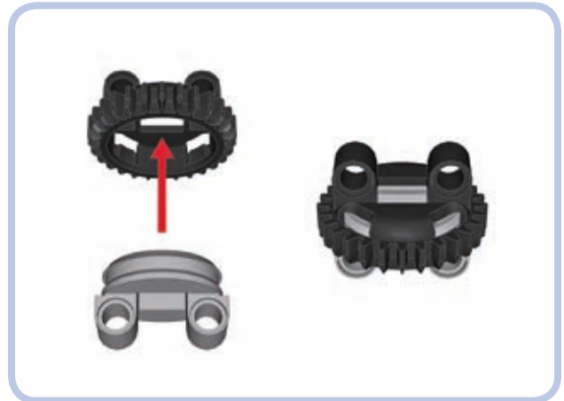
Figure 5-23: A small turntable consists of two halves
