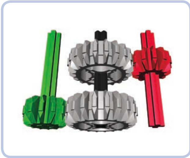
Figure 5-6: The middle gears in this picture are idler gears. Both are meshed with only one gear, but they are mounted on the same axle and are of exactly the same size, which means that they work just as a single gear would.
