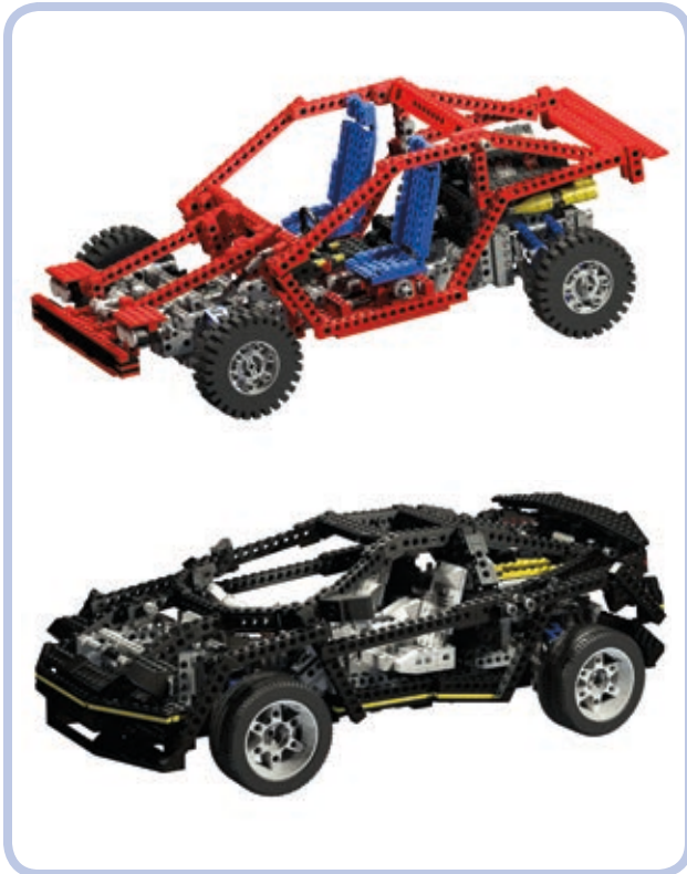
Figure 14-16: The LEGO 8865 and 8880 sets are designed with Ackermann geometry in mind.
