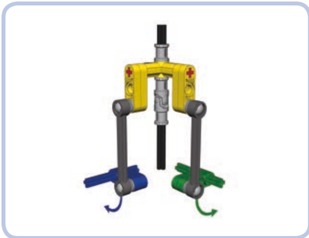
Figure 19-22: A mechanism for tilting a rotor in two planes. Rotating the green axle tilts the rotor in one plane—for example, forward and backward—while rotating the blue axle tilts the rotor in another plane—for example, left and right. Thanks to the use of links and towballs, both angles of the rotor can be changed simultaneously without interference.
