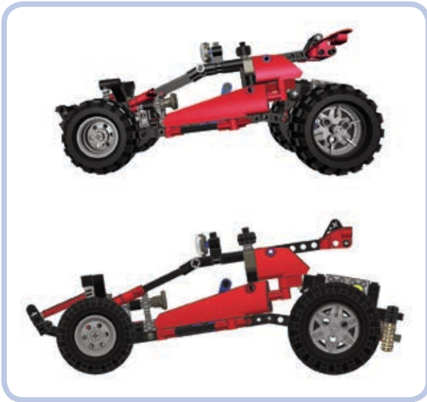
Figure 20-2: Side view of the same model with central perspective (top) and without central perspective (bottom)
