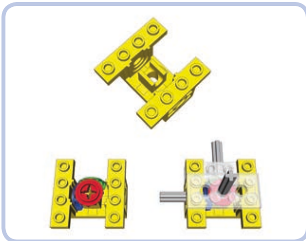
Figure 11-19: Piece #6585 is a particularly interesting brace that can reinforce both horizontal and vertical gears. Technic bricks and plates can be connected to it to support their axles.
