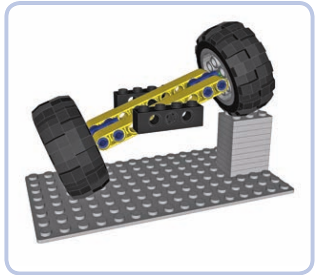
Figure 15-15: A pendular suspension negotiating an obstacle with one wheel. Note that the chassis, which is connected to the axle by the axle going through its center, is raised by 50 percent. This is generally bad for stability and for the driver's comfort.
