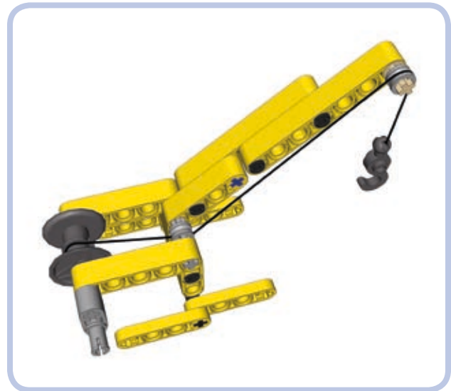
Figure 6-14: A simple crane uses a winch to pull a load on a hook up and down. The movement is transferred through a string, which is guided from the reel to the top of the crane by two half bushes acting as idler pulleys.
