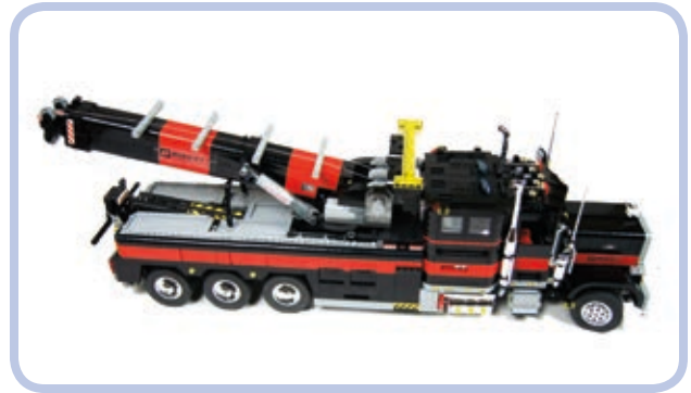
Figure 21-4: My tow truck model housed 17 motors and nearly 19 meters of electrical wires, requiring ducts inside the body. Note that the mechanical and electrical parts are all enclosed within the body, with a few minor exceptions, such as the PF Medium motor, which is partially visible by the boom's winch, and the gears of the steering system, which are visible next to the front mudguard.
