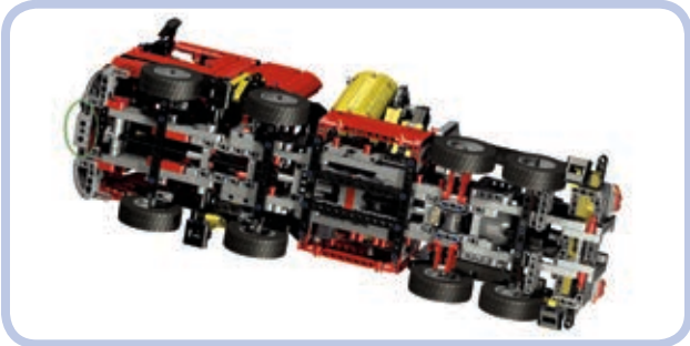
Figure 3-23: The 8285 Crane Truck set is an outstanding achievement in creating a rigid, sturdy studless chassis for a heavy vehicle. Studfull pieces are still there—note the clever use of a Technic brick to attach the license plate under the front bumper.
