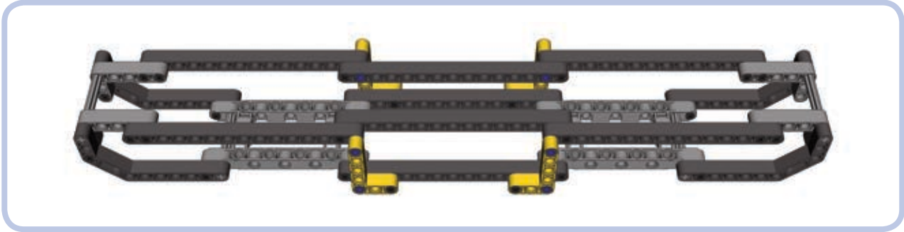
Figure 11-32: A studless body frame with two pairs of rails, one above the other. The upper pair is supported at the ends and in the middle. Studless frames work well with smaller, compact models where adding many elements to the chassis is more important than its rigidity.
