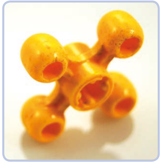
Figure 11-54: This visibly worn knob has polished edges where the material has been rubbed away. Knobs transfer high torque over very small areas of contact, resulting in intense wear. Worn knobs produce a distinctive squeaking when working under stress.
