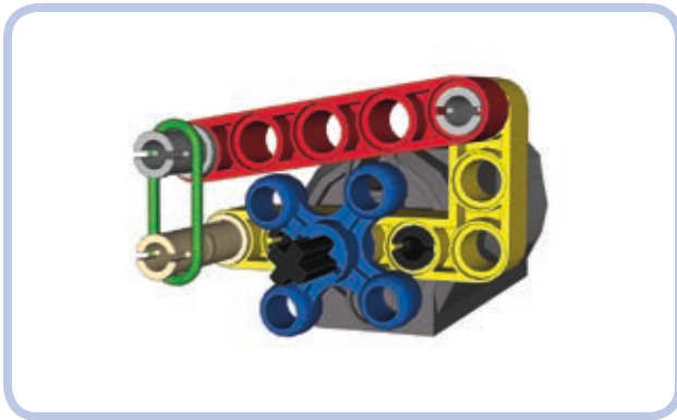
Figure 8-20: The knob on the motor's output axle (blue) has a beam (red) fastened to it at all times by a rubber band (green). This makes a regular motor behave similarly to a stepper motor.
