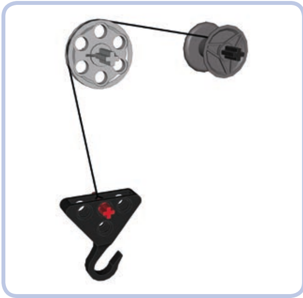
Figure 6-16: This arrangement has an upper group with a single pulley and no lower group. The string that comes off the pulley is tied directly to the hook. No pulley system is created, and no mechanical advantage is gained.
