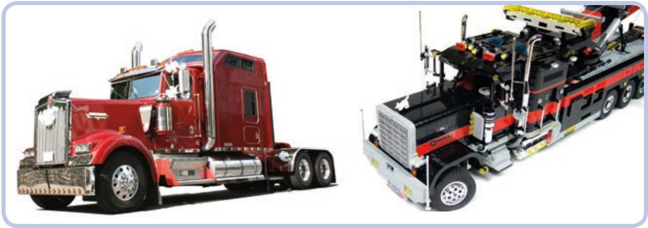
Figure 21-13: Because of their unrealistic steering geometry, LEGO wheels need more spacious mudguards than real wheels do. If the mudguards of my tow truck weren't sized up relative to the real ones, the wheels would collide with them.
