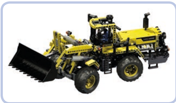
Figure 7-11: The LEGO 8265 set features a complex front loader whose arms (elevating the bucket) form parallel levers.
