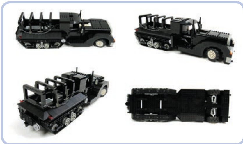
Figure 19-13: My model of a half-track truck. Vehicles of this type are driven by tracks and steered by front wheels.
