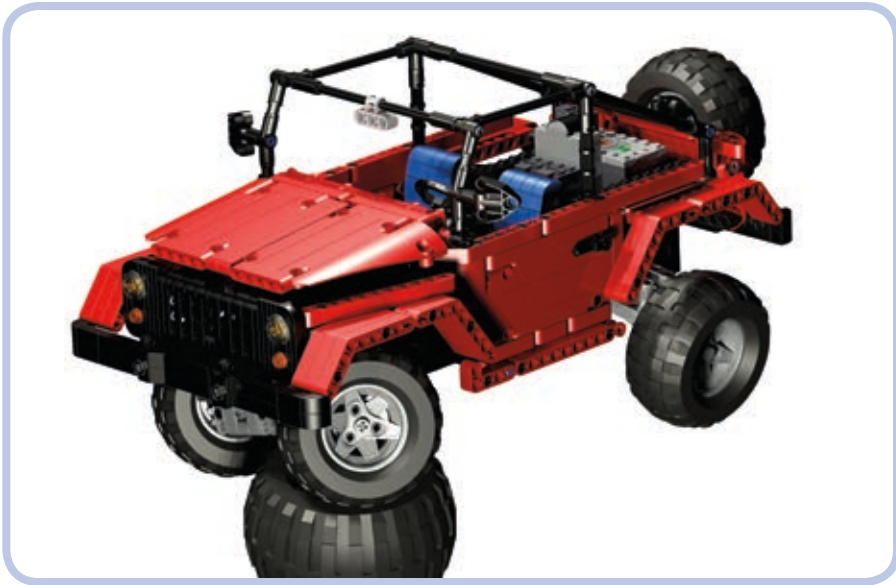
Figure 19-3: My model of the Jeep Wrangler Rubicon, which is a small open-top car, had motors under the hood and the battery and IR receiver in the trunk. This way it had a good weight distribution and plenty of space left for some decorative elements in the cabin interior, including seats and the steering wheel.
