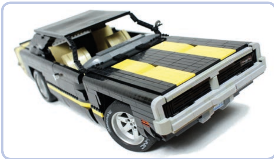
Figure 19-1: My 1969 Dodge Charger model appears to have a massive hood with plenty of space beneath it. However, since I decided to model the car's huge engine, almost none of this space was available for mechanical components, and I was barely able to fit a mechanism to lift the distinctive grille that reveals the car's headlamps. Most of the electric components ended up in the trunk.
