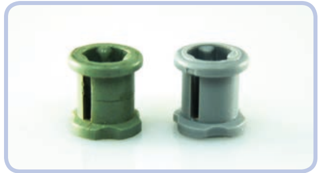
Figure 11-49: A bush: roughly 20 years old (left) and 1 year old (right). Note the crack in the old bush's side; under torque, this crack will soon lead to the bush's disintegration.
