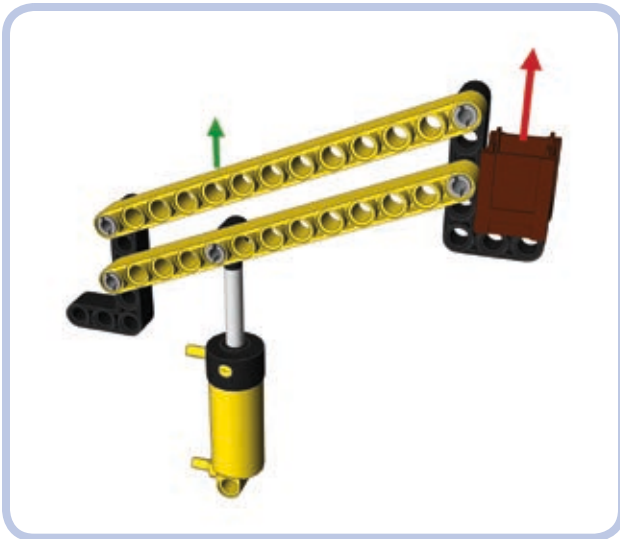
Figure 7-10: A boom of a crane made of parallel levers. The parallel levers ensure that the element on the end of the levers maintains constant orientation as the levers move it up and down.
