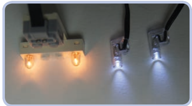
Figure 8-26: A 1x4-stud 9V brick with lights (left) and a pair of Power Functions LED lights (right). Note the difference in the color and direction of the light.
