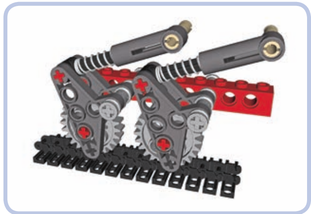
Figure 16-23: A more complex trailing arm system that works with 24-tooth gears
