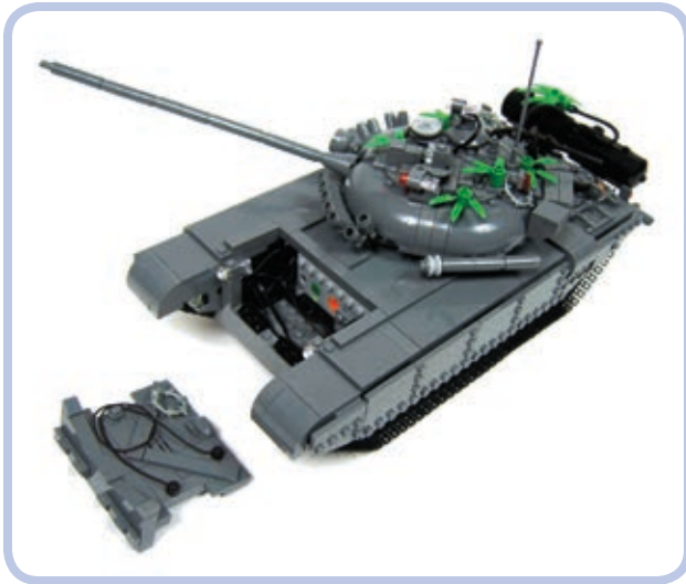
Figure 19-11: My T-72M tank model was small and low, with an angled glacis plate that left very little space in the front of the hull. The very front of the hull housed only some wires, and the glacis plate was removed to access the battery.
