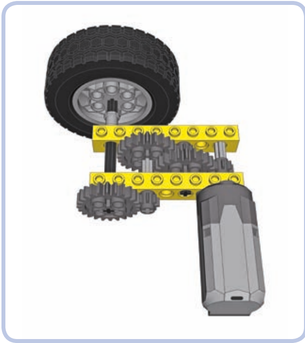
Figure 11-5: The two pairs of 1x4 bricks from our original structure have been replaced with two single, solid 1x8 bricks.
