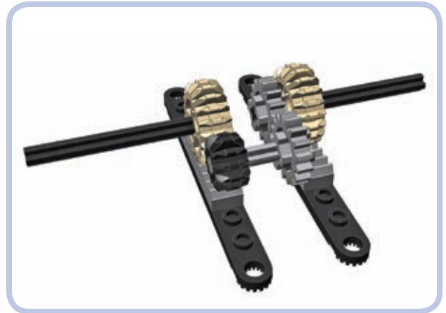
Figure 14-26: Second method for two axles with different steering locks: two identical pinions but two separate steering shafts with gearing between them
