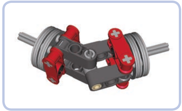
Figure 8-36: A custom universal joint is more robust but also larger than ready-made ones.
