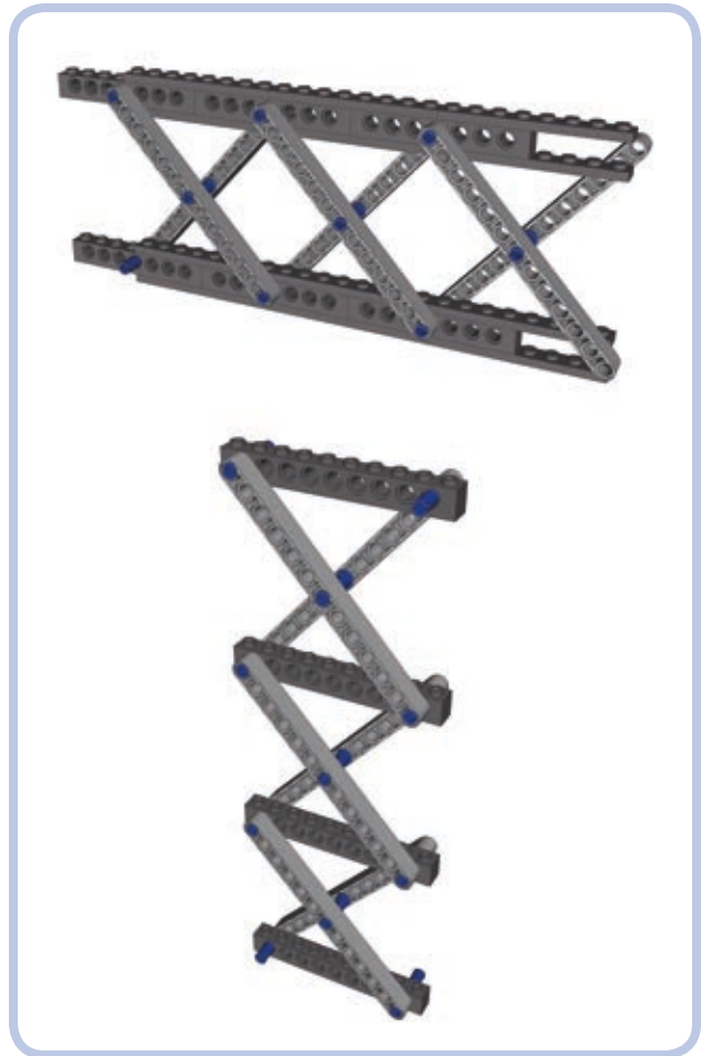
Figure 11-40: Planar combinations of the Brown truss module
