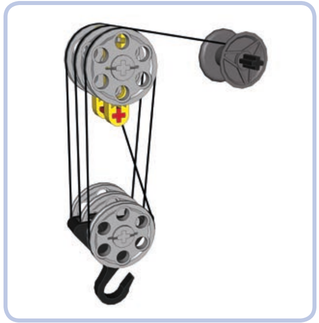
Figure 6-21: This system, called threefold purchase, grants a mechanical advantage of 6.
