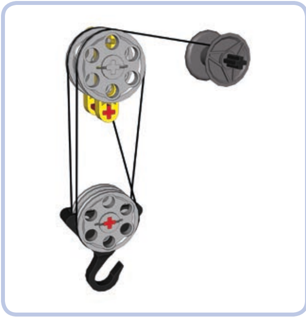
Figure 6-19: This system, called double tackle, grants a mechanical advantage of 4.
