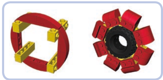
Figure 21-15: Two circular structures built with small basic pieces. One is built around bricks with studs on the side, and the second is built with hinge plates embracing a tire. Both are prone to disintegration if sufficient stress is applied.
