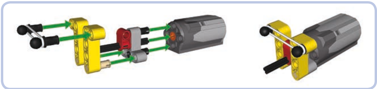
Figure 14-12: The rubber band-based return-to-center steering attachment for a PF Medium motor
