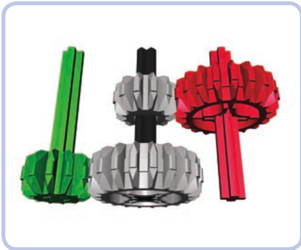
Figure 5-7: The middle gears in this picture are not idler gears. Both are mounted on the same axle, but they are of different sizes, which means that they affect how torque and speed are transformed. This is because the varying size of the gear affects the torque it transfers.
