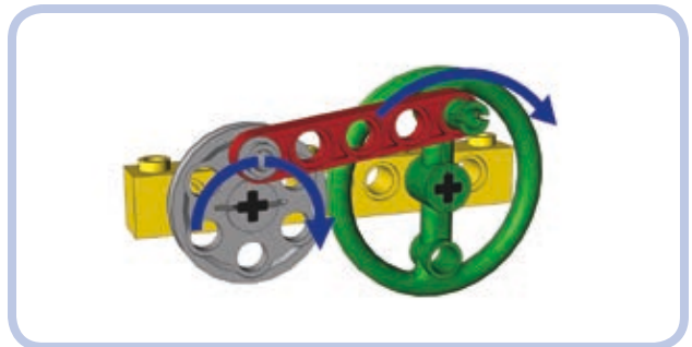
Figure 8-13: An eccentric mechanism with two discs connected by a beam. The smaller disc makes full rotations, and the larger disc makes only partial rotations back and forth.
