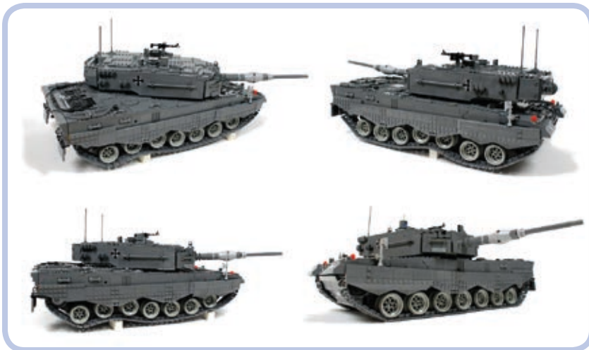
Figure 19-12: My model of the Leopard 2A4 tank was large and heavy. I used four XL motors for propulsion, powered from two battery boxes located in the middle of the hull. It wasn't fast, but it had plenty of torque and handled obstacles extremely well for its weight.
