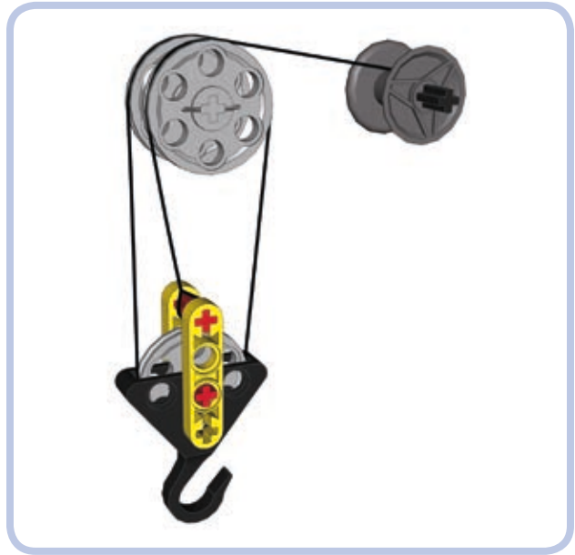
Figure 6-18: A pulley system with three sections of string between the groups. The upper group has string coming through it twice and hence two pulleys to prevent the string from getting tangled up. The string is then tied to the red axle in the lower group. This arrangement grants a mechanical advantage of 3.
