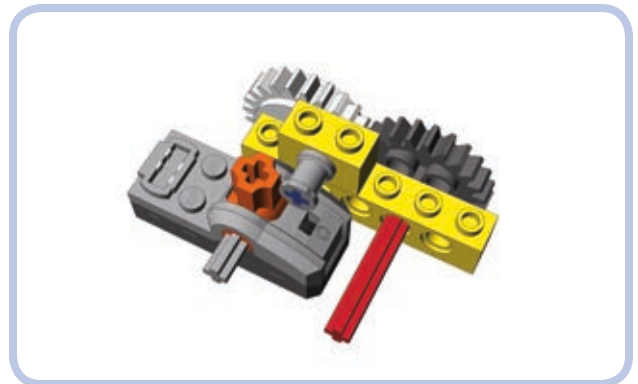
Figure 8-23: A blocked Power Functions switch is connected to a vehicle's driveshaft (red) through a 24-tooth gear with clutch (white).
