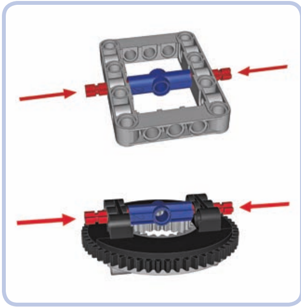
Figure 11-23: Dangerous structures: Once the axles marked by arrows are pushed in, these structures are impossible to take apart without cutting pieces.
