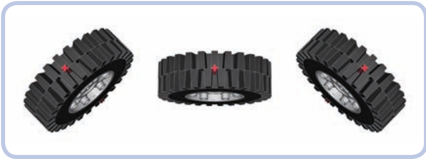
Figure 21-9: The steering geometry of a real vehicle's wheel: As the wheel is steered, it rotates around a pivot point going through its center, marked in this series of images by an "imaginary" red axle.
