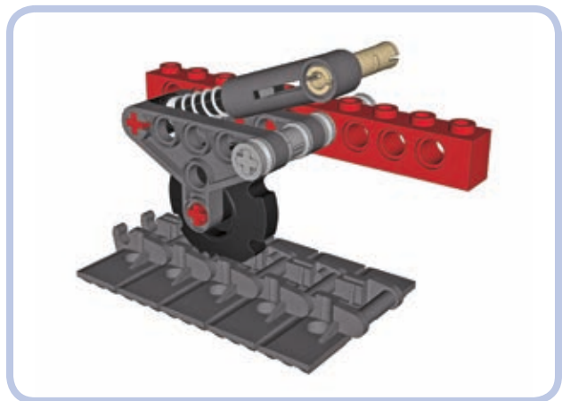
Figure 16-24: Another compact trailing-arm setup
