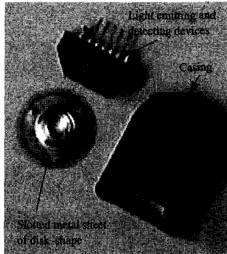
Fig. 5.41 Picture of a dismantled incremental optical encoder.
