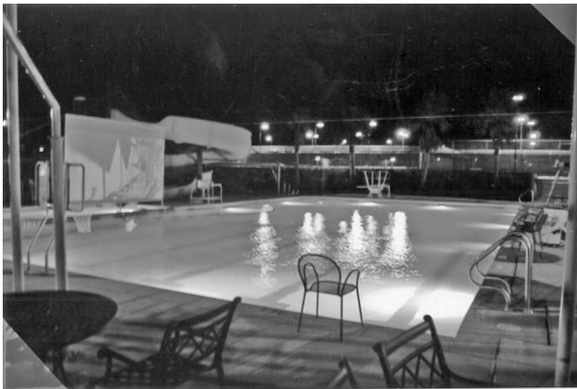
FIGURE 5.4 An insufficiently illuminated pool.
