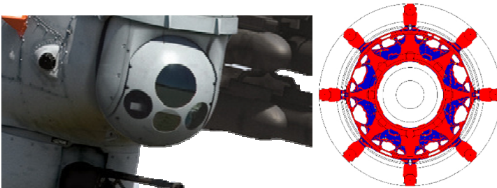
Figure 7.5. A helicopter aiming system and shape-preserving design of its pedestal
