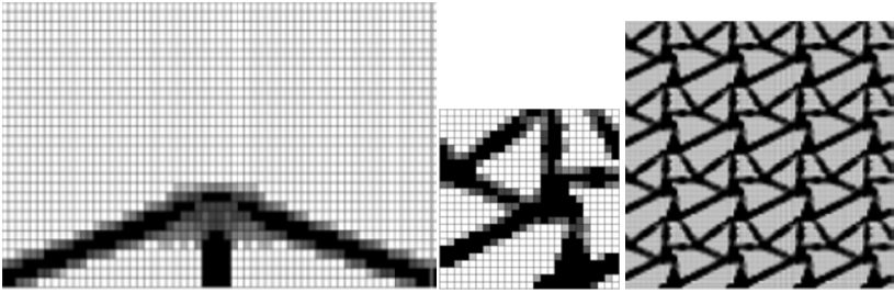
Figure 1.22. Simultaneous topology optimization of microstructures and macrostructures [YAN 08]
