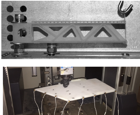
Figure 7.11. Loading test with stereolithography resin model of additive manufacturing
