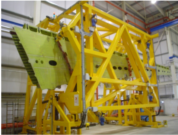
Figure 7.4. A typical assembly jig for aircraft wing
