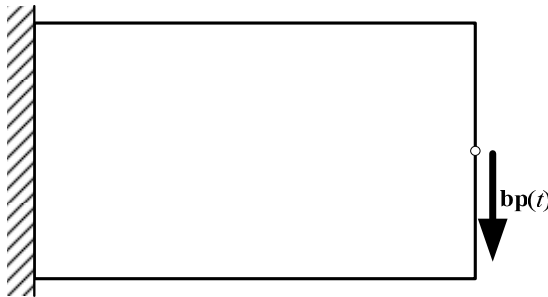
Figure 3.16. 2D cantilever beam (800 plane elements, 1,722 DOFs)
