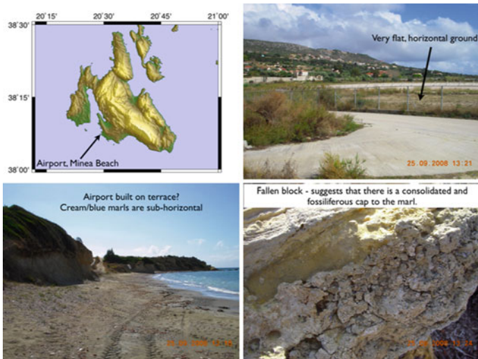
Fig. 9.13 The airport is built on a wide, flat plain ~ 10m above sea-level. The limestone bedrock outcrops in small patches on the headlands, where it dips ~ 45° to the SW. Everywhere else, the flat region is underlain by subhorizontal yellow and blue marls. Although the top of the surface is heavily tarmaced and vegetated, fallen blocks on the beach were suggestive of a recent marine cap, containing corals, L. lithophaga and shell fragments. The top of the marls certainly looks like an erosional feature, suggesting that the airport is built on a marine terrace
