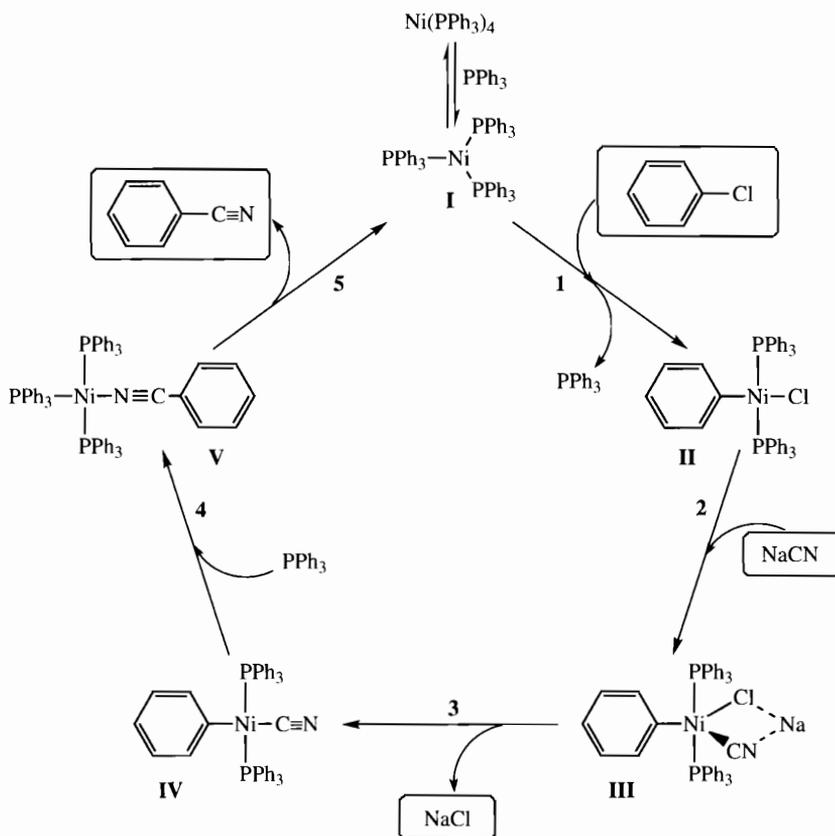
Fig. 1. Mechanism of  $\text{Ni}(\text{PPh}_3)_4$ -catalyzed cyanation of chlorobenzene
