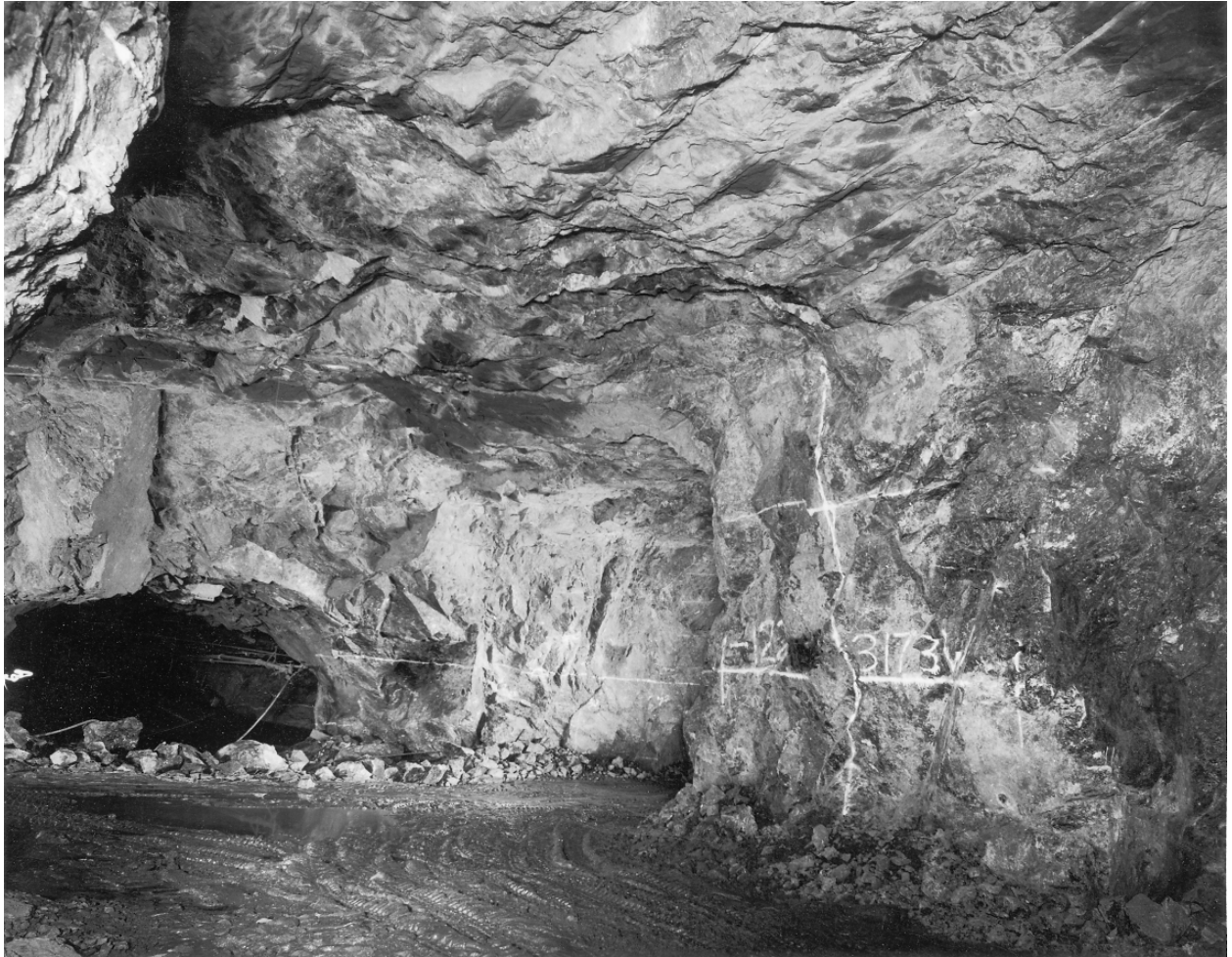
Frontispiece Post-pillar mining in a jointed and faulted rock mass at the Dolphin Mine, King Island, Australia (photograph by permission of King Island Scheelite and CSIRO Division of Geomechanics).
