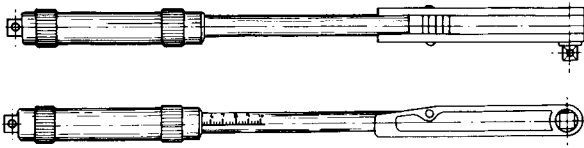
Figure 3.76 Torque spanner (wrench) for use with sockets
