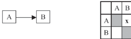
Fig. 2.1-8 Example of link representation in network form and matrix form
