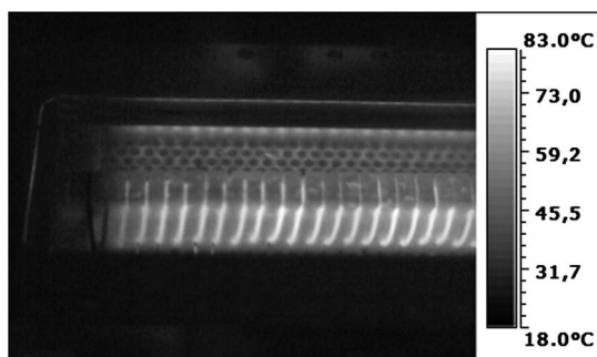
Figure 4.14 Thermographic image (SP Thermoview 8300) of the tube surface with an n -propanol/propionic acid reactant mixture heated in it. The experiment was run with a continuous flow of reactants at a 0.5 \text{ ml min}^{-1} flow rate and a microwave power of 80 W. The microwave power was stopped and the lid on top of the cavity was opened to view the temperature development inside with the thermal camera. This configuration enables heating up to the boiling point of the liquids.
