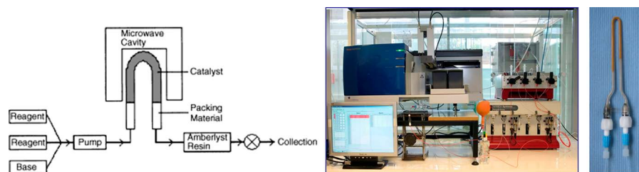
Figure 1.12 Experimental set-up for a Suzuki coupling catalysed by PdEnCat. Reproduced from ref. 62 with permission.
