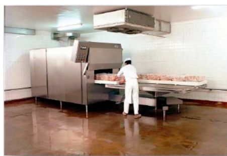
Figure 3.13 Tunnel for tempering, thawing and defrosting of meat blocks. 72 Reproduced with kind permission of Sairem SAS – http://www.sairem.com/ .
