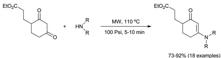
Scheme 1.7 Solvent- and catalyst-free synthesis of \beta -aminoesters under MWI.
