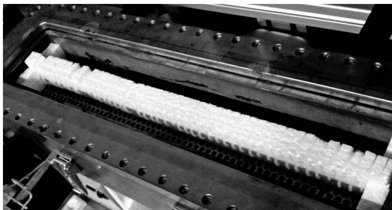
Figure 4.13 Spiral flow configuration in TE_{10n} cavity. A thin tube is wound around an expanded polystyrene placeholder. As such a configuration is created with a relatively large portion of tube length that is oriented vertically, parallel with the electric field vector of the microwave field supported in the cavity.
