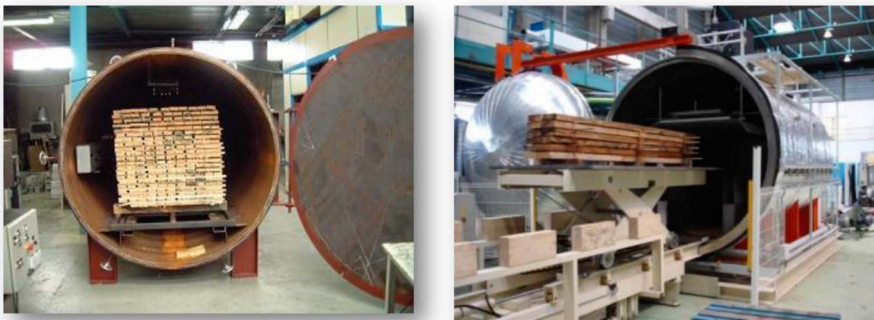
Combined 50 kW, 27.12 MHz & steam pressure (2 bars)
