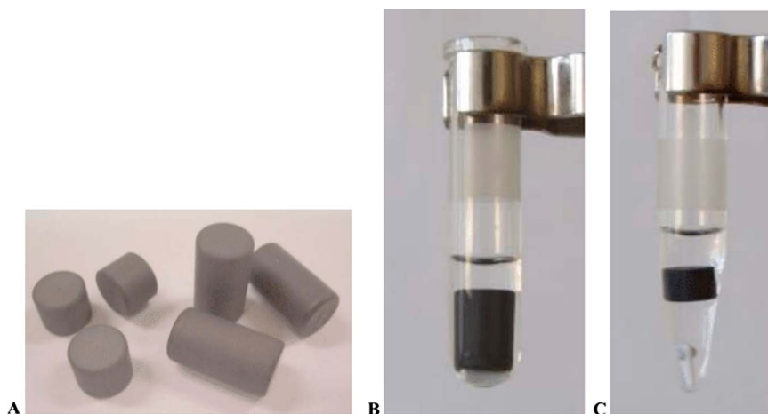
Figure 1.4 (a) SiC cylinders: 10 × 8 mm (1.94 g) and 10 × 18 mm (4.35 g). (b) SiC cylinder (10 × 18 mm) inside a standard 10 mL microwave vial used in single-mode microwave apparatus, solvent volume 2 mL. (c) SiC cylinder (10 × 8 mm) inside a standard 5 mL conical microwave vial, solvent volume 2 mL. Reproduced with permission from J. M. Kremsner and C. O. Kappe, J. Org. Chem. 2006, 71, 4651–4658. Copyright (2006) American Chemical Society. 30
