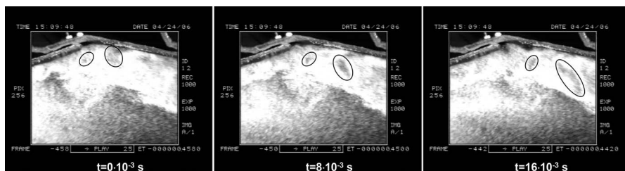
Figure 12.8 Bubble formation and motion in an RFB-SG visualized by means of a high speed CCD camera at 1000 \text{ frames s}^{-1} focusing on the vicinity of a single gas inlet slot. Vortex chamber design: see Figure 12.2. Total gas flow rate: 0.2 \text{ m}^3 \text{ s}^{-1} , solids loading: 1.1 \text{ kg} , 300 \mu\text{m} alumina particles. (From De Wilde.) 32
