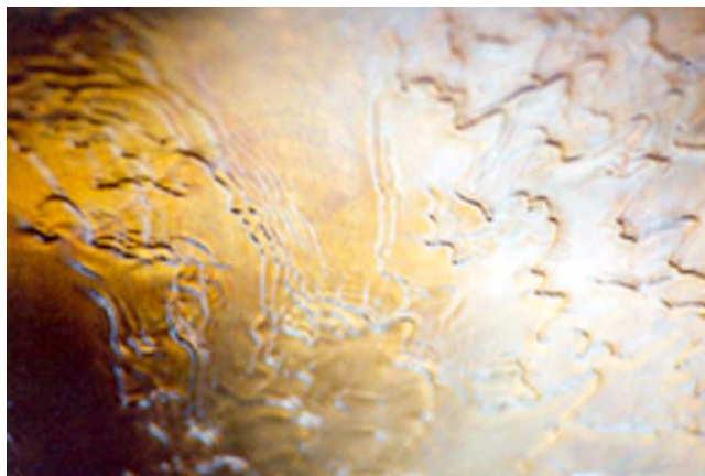
Figure 11.2 Thin, wavy film flow on a rotating disc. (Reprinted from ref. 1 ©2013 John Wiley & Sons.)
