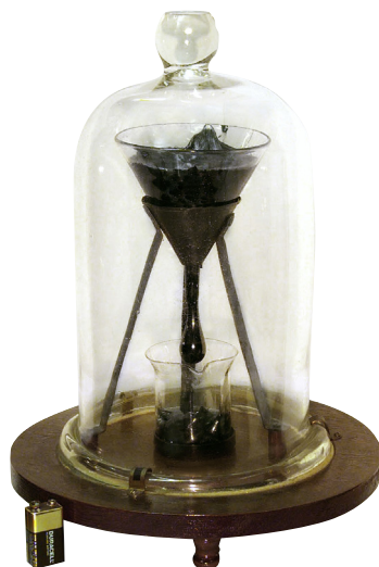
Figure 3.2 University of Queensland pitch drop experiment showing the viscoelastic nature of pitch.
