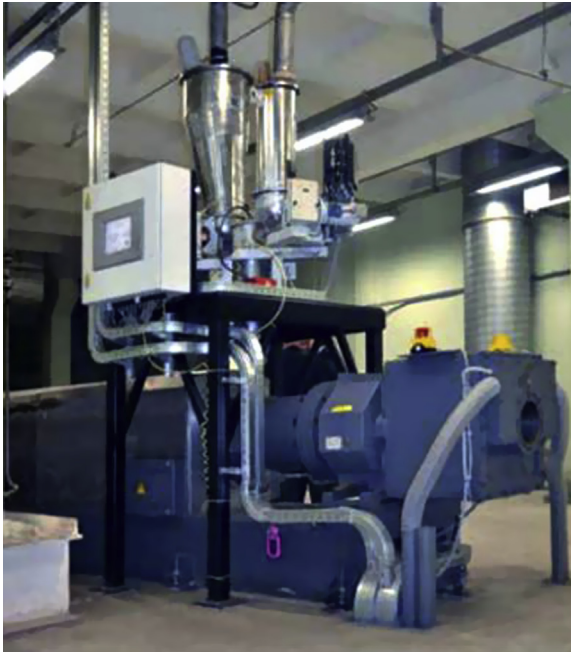
Figure 9.22 Extruder with gravimetric dosing system in SymTTec. Reprinted from Truetzschler, Man-made Fibers. [Online]. Available: http://www.truetzschler-manmadefibers.com/fileadmin/user_upload/truetzschler-nonwovens/brochures_downloads/man-made-fibers/englisch/MMF_EN.pdf with permission of Truetzschler.
