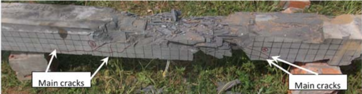
H8A specimen with 1000 kN axial load under 24 kg charge weight loading
