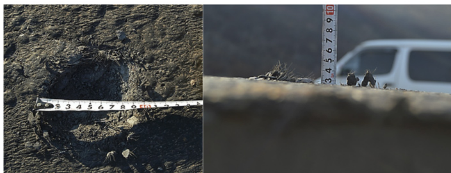
Top surface concrete crater diameter and depth
