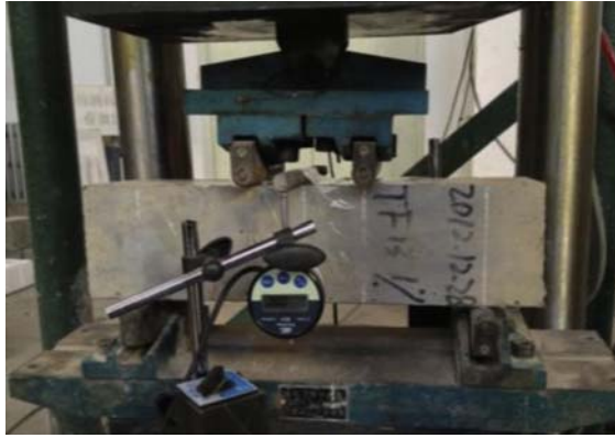
Figure 2.3 Setup of the flexural tests.
