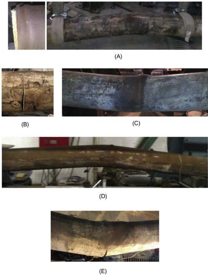
Figure 5.43 Failure modes of circular specimens: (A) C1A, (B) C2A, (C) C2B, (D) C3A, and (E) C3B.
