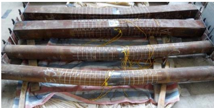
Figure 5.9 Overall deformed shapes after residual capacity test.
