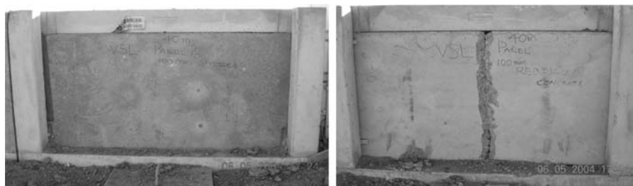
Figure 1.7 UHPC slab versus NSC slab under 5 ton Hexolite-RDX/TNT detonation at 40 m standoff distance.
