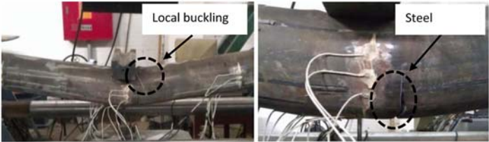
Figure 5.32 Failure mode of TPB_C1.
