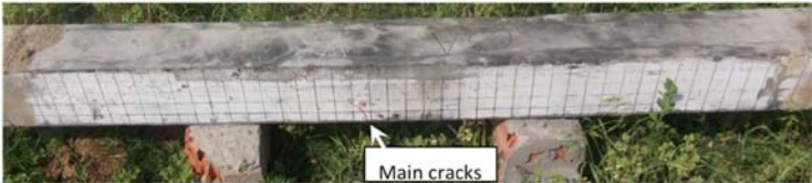
U6B specimen with 1000 kN axial load under 24 kg charge weight loading
