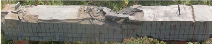
H8B specimen with 1000 kN axial load under 8 kg charge weight loading
