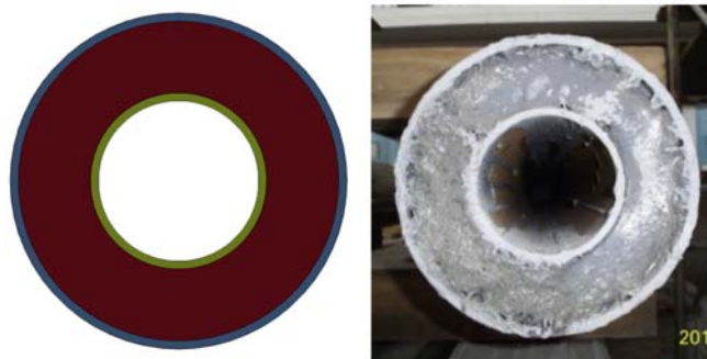
Figure 5.63 Circular cross-section of the numerical model (left) and the actual column (right).
