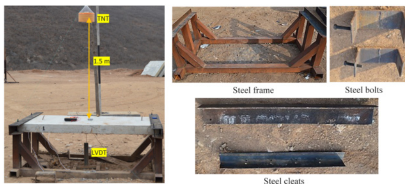
Figure 3.82 Close-in detonation setup and clamping system.
