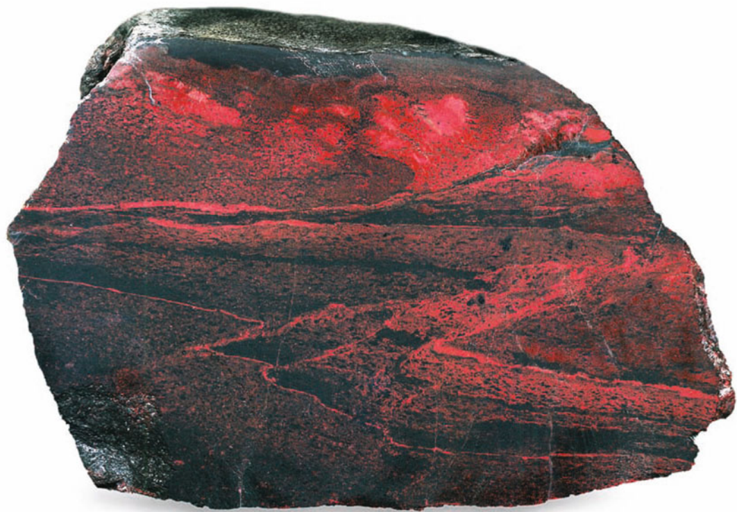
Sedimentary ore from the Skonca beds with laminated cinnabar layers in black Langobardian shale. Skonca beds were named by Lipold (1874) after the creek Skaunca (today Skavnica), where he found outcropping shales, which contain a rich syngenetic mineralization with cinnabar in the ore deposit not far from the creek. 11 x 8 cm. Find J. Čar. Collection of the Municipal Museum of Idria – Photo: A. Zelenc
