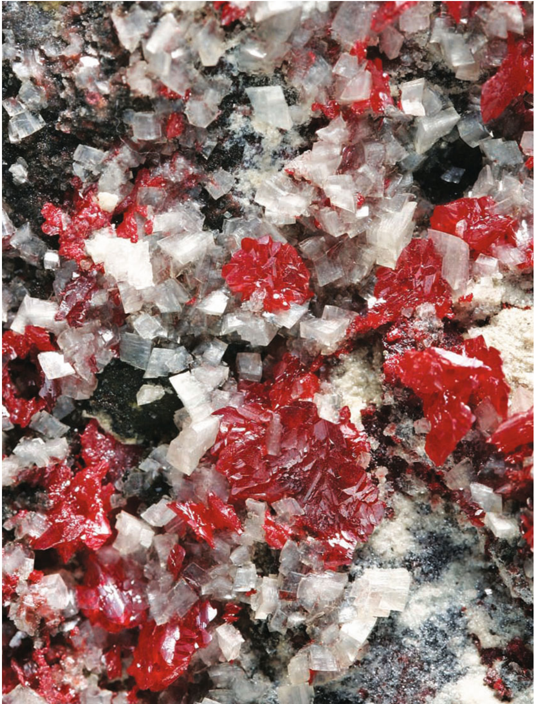
White dolomite crystals intergrown with up to 2 mm large rosettes of cinnabar composed of several crystals slightly rotated with respect to each other. The reason for such growth is not known. The specimen dates back to 1900. Collection J. Zavašnik – Photo: A. Rečnik
