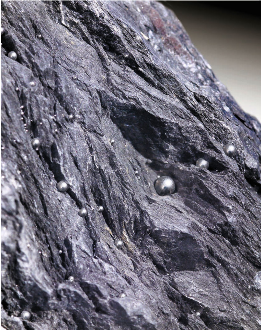
Native mercury in Carboniferous slate from the mining field Karbon on the III rd level. In Idria, mercury was originally discovered in the same type of host rocks, which are constituting the overlying beds of the ore deposit. In the slate mercury is dispersed in the form of microscopic droplets that condensate into larger drops on the exposed outcrops. Because of their specific weight they quickly slip and disappear in the ground. Overall specimen size 15 cm, detail 6 cm. Collection of the Municipal Museum in Idria – Photo: A. Rečnik
