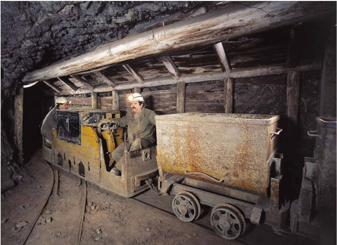
Electric train used for transportation of ore to the shafts, where it was loaded on elevators and lifted to the surface. After shutdown, this became a part of the technical heritage – Photo: B. Kladnik
