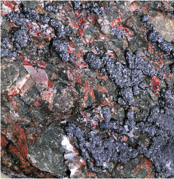
Compact layer of pitch black metacinnabar crystals on the surface of mineralized limestone-dolomitic conglomerate from the Lamberg-Ruda mining field on the IX th level. The host rock is cemented by cinnabar, which was probably the main source of mercuric sulfide for crystallization of metacinnabar in freshly opened fissures. Unaltered metacinnabar is considered a rarity. Shown is a 35 mm detail from a 13 cm specimen. Mineralogical collection of the Municipal Museum of Idria – Photo: A. Rečnik
