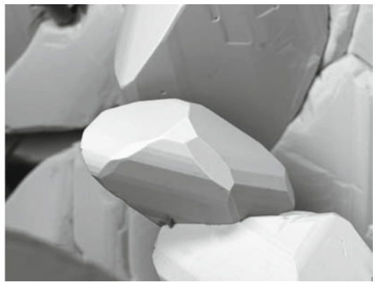
Form-rich cinnabar crystal from a small cavity in Lower Scythian dolomite on IX th level. The crystal habit is defined by a flat rhombohedron truncated by pinacoid. Further it is modified by a series of rhombohedral faces, a hexagonal prism and a trigonal bipyramid. Crystal size 60 \mu\text{m} – SEM Photo: A. Rečnik
