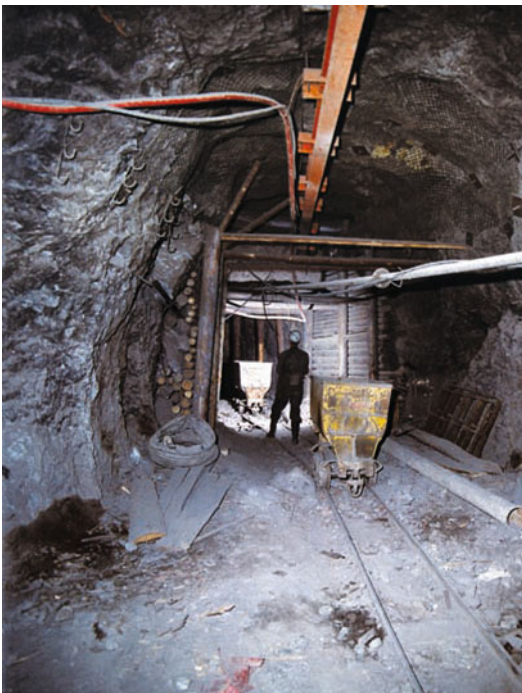
Electric train used for transportation of ore to the shafts, where it was loaded on elevators and lifted to the surface. After shutdown, this became a part of the technical heritage – Photo: B. Kladnik
