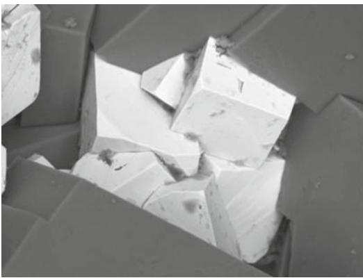
A cluster of simple rhombohedral crystals of cinnabar, partly overgrown by dolomite crystals from IX th level. Simple crystals like this are not common. They belong to an older generation of cinnabar that grew relatively rapidly from saturated solutions. The size of the detail is 100 \mu\text{m} – SEM Photo: A. Rečnik
