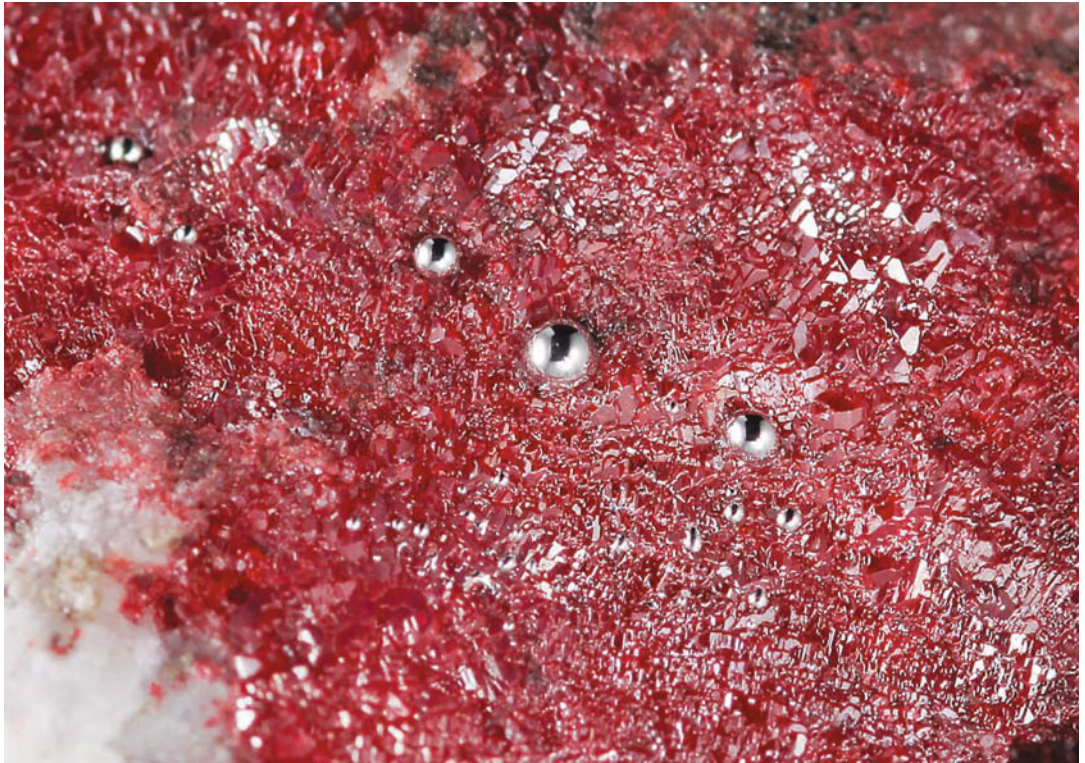
Fissure in oolitic limestone richly mineralized with cinnabar, calcite and native mercury. The fissure was originally filled with crystalline calcite. After intrusion of hydrothermal solutions calcite was metasomatically replaced by cinnabar to some extent. This was followed by a further extension of the fissure with the empty space being filled by dilute, oxygen-rich solutions. On freshly opened surfaces cinnabar recrystallized by forming many small facets in identical orientation to the primary cinnabar grain, while some cinnabar was reduced to native mercury. The droplets of mercury on a 6 cm specimen measure up to 1 mm. Collection V. Pavčić – Photo: A. Rečnik
