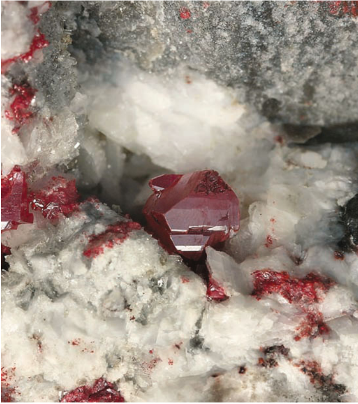
Simple rhombohedral crystal of cinnabar with quartz crystals in a calcite-lined cavity. Primary rhombohedral form is modified by flat rhombohedra and a rugged pinacoidal face. Size 4 mm. XI th level, Delo shaft. Find and collection J. Klemenčič – Photo: A. Rečnik
