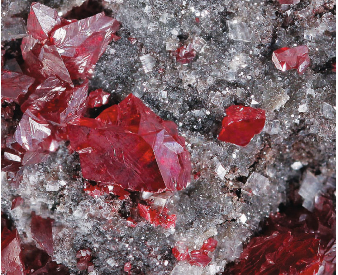
Cinnabar is the main ore mineral in Idria. It occurs as a massive ore or in the form of face-rich crystals with adamantine to submetallic luster. At elevated temperatures mercuric sulfide forms two polymorphic modifications, cubic metacinnabar and hexagonal hypercinnabar. Metacinnabar is well known in Idria, whereas hypercinnabar has not yet been determined in this ore deposit. Photograph shows ruby-red crystals of cinnabar on dolomite. Detail 12 mm. Collection of the Faculty of Natural Sciences in Ljubljana – Photo: A. Rečnik
