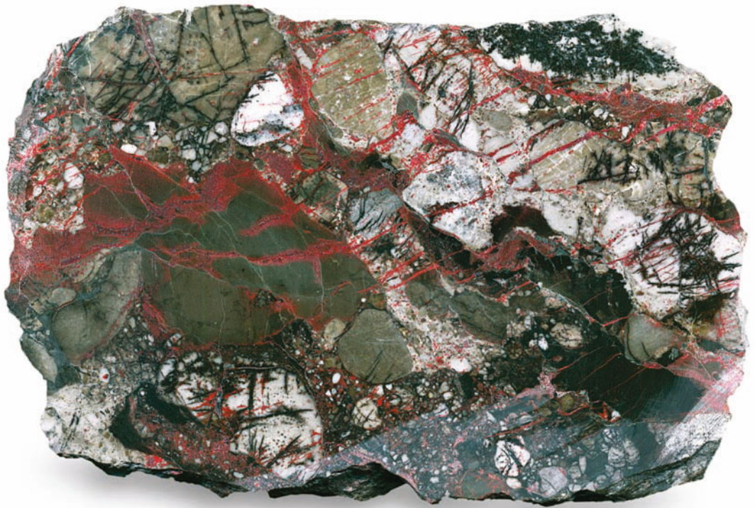
Langobardian dolomitic conglomerate is composed of poorly sorted white and grey dolomite clasts mineralized with cinnabar, pyrite and bituminous matter filling fissures and pores of the tectonically shattered rock. The specimen of brecciated cinnabar ore originates from the Skonca beds. Size 15 x 10 cm. Geological collection of the Municipal Museum in Idria – Photo: A. Zelenc
