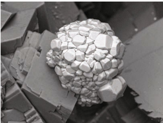
Cluster of framboidal pyrite on dolomite. This form of pyrite is typical for crystallization from colloidal solutions in the presence of hydrocarbons. Ore body Grüberler, XIII th level. The width of the photograph is 50 \mu m – SEM Photo: A. Rečnik
