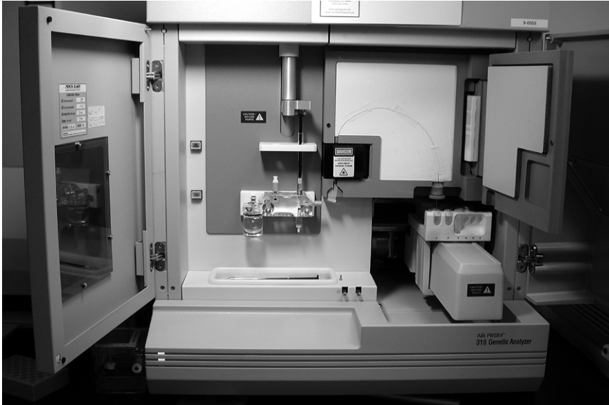
Figure 6.19 ABI PRISM® 310 Genetic Analyzer. In forensic science, this instrument is used for the automated analysis of length polymorphisms, primarily STRs, and for mitochondrial DNA sequence analysis. A capillary column filled with liquid acrylamide polymer is used to separate fluorescently labeled fragments that are detected with a laser as they run past a predetermined point. The computer software then assists with data analysis and allelic typing. (Courtesy of Serological Research Institute.)
