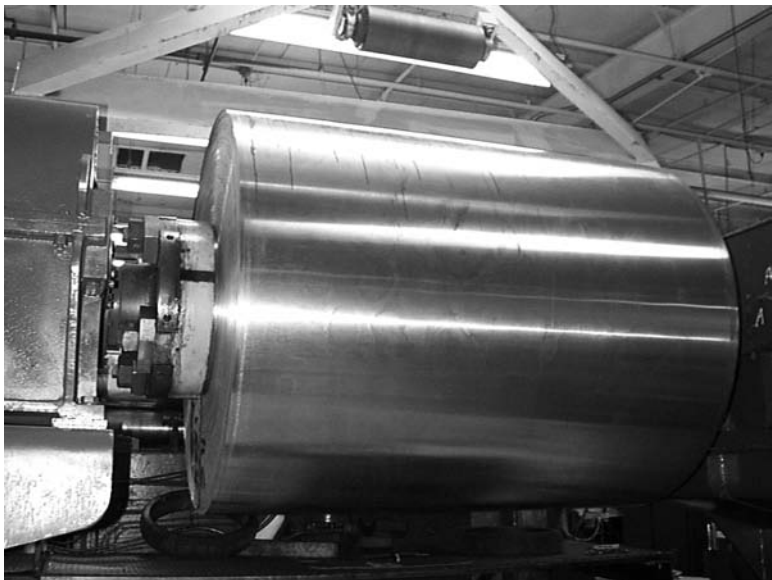
12.28 Photograph of a coil of AA5083 materials exhibiting dirt/debris streaks on the coil which must be removed to ensure proper paint application.
