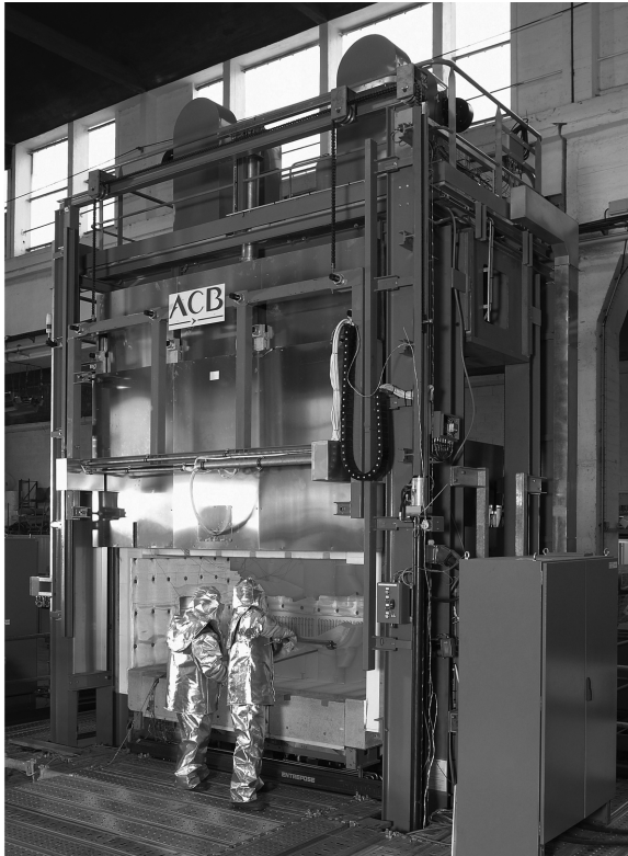
3.5 Standard SPF four-column press-furnace with manual blank removal after SPF (courtesy ACB-PS, www.acb-ps.com ).
