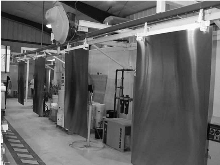
12.27 Blank lubrication conveyor. Blanks are hung on a conveyor and then processed through a wash station, heater, and robotic paint sprayer to apply the lubricant.
