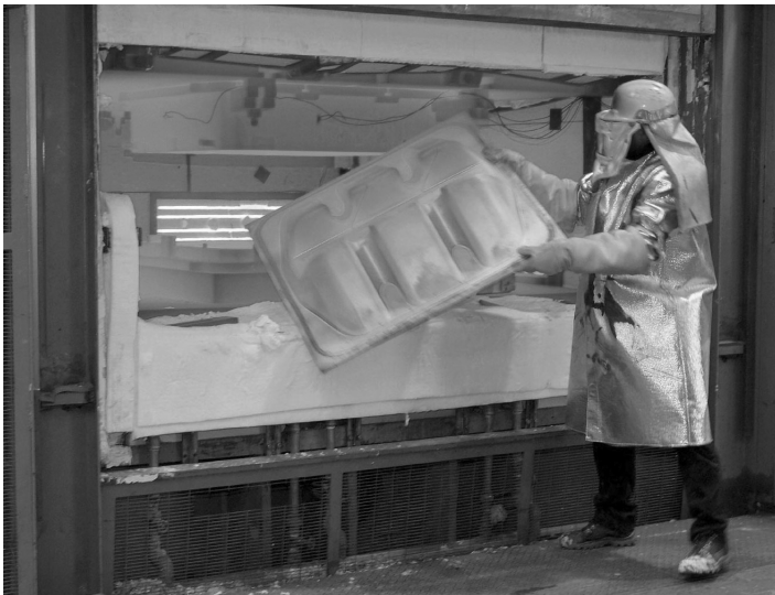
10.13 A 4-part SPF Ti pressing (copyright Aeromet International plc).
