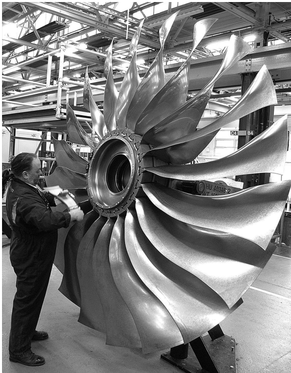
10.11 Ti-6Al-4V hollow, wide-chord fan blades on a Rolls-Royce Trent series gas turbine engine (copyright Rolls-Royce plc).
