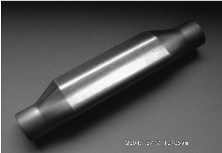
3.2 Hollow cavity SPF forming: steel tube after SPF (courtesy FormTech GMBH, www.formtech.de ).
