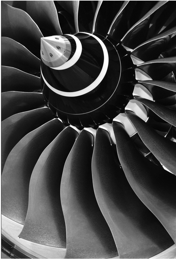
10.1 Ti-6Al-4V hollow, wide-chord fan blades on a Rolls-Royce Trent series gas turbine engine (copyright Rolls-Royce plc).
