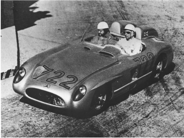
13.1 1955 Mercedes Benz 300 SLR racing car. The body panels were fabricated from magnesium sheet.
