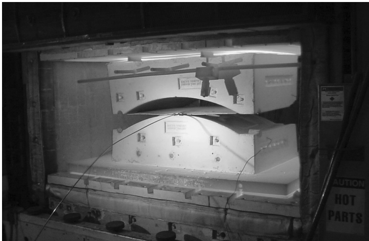
3.12 Ceramic die reinforced with fused silica rods for TA6V aeronautic parts forming (courtesy Dan Sanders, Boeing Company).
