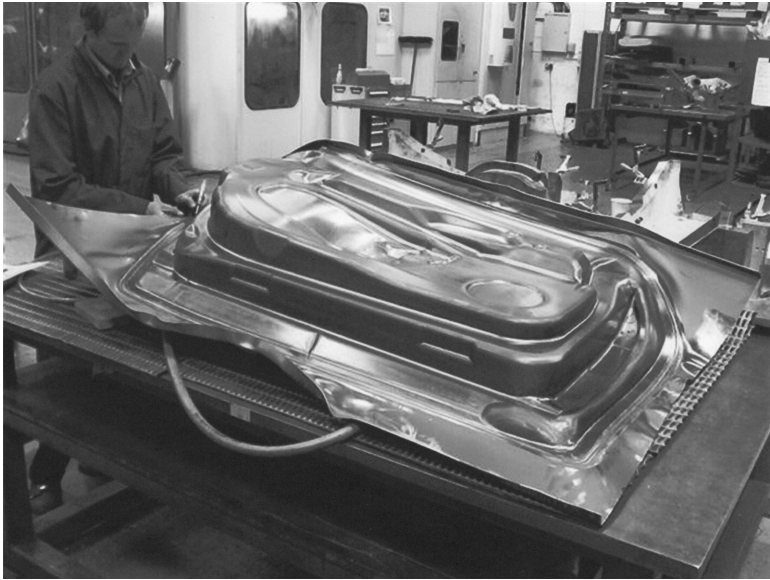
13.5 Trial pressing of inner door panel in AZ31B (courtesy of Superform Aluminium).
