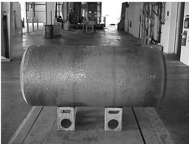
10.5 Vacuum arc remelted titanium ingot (copyright Timet).
