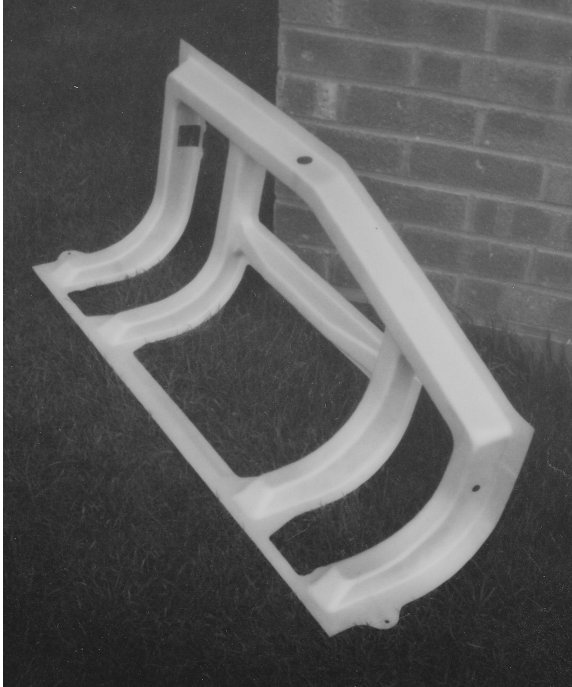
11.3 Inner structure of military aircraft door superplastically formed from the Al-Li based alloy AA8090.
