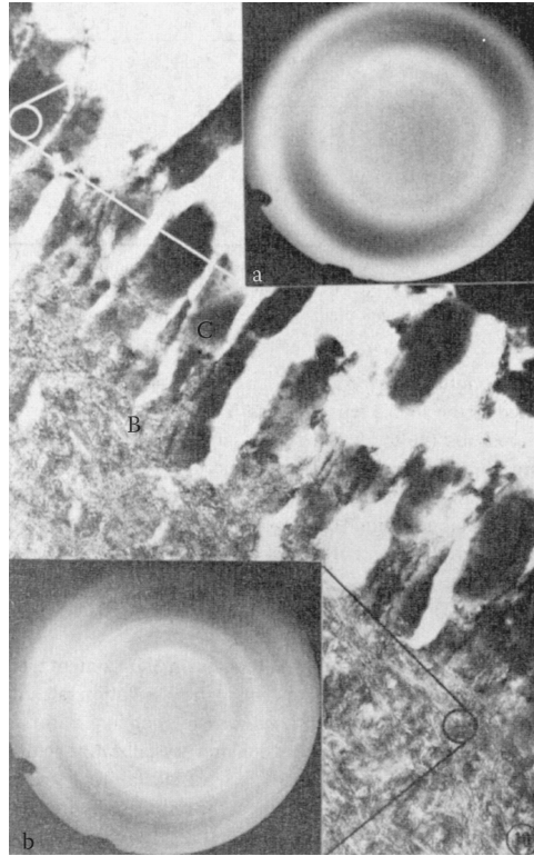
FIGURE 29.15 Transmission electron micrograph of well-mineralized bone (B) juxtaposed to the glass-ceramic (C) which fractured during sectioning ( \times 51,500 ). Inset (a) is the diffraction pattern from ceramic area and (b) is from bone area. (From Beckham C.A., Greenlee T.K. Jr, and Crebo A.R. 1971. Calc. Tiss. Res. 8:165–171. With permission.)
