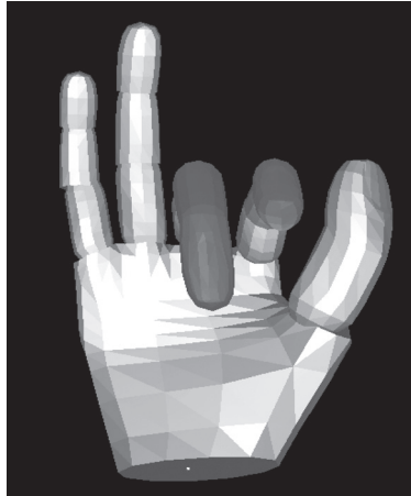
FIGURE 53.12 Cyber hand with digits was developed and the digits moved under the control of single units by subject JR.
