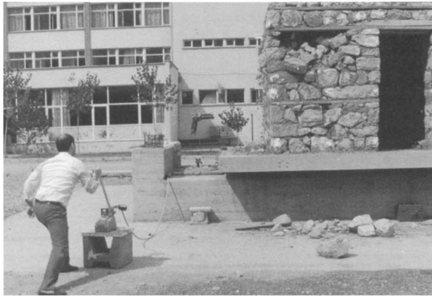
Figure 8.3 Testing full-size strengthened stone masonry houses on the Ankara impulse table (from Andrew Coburn).
