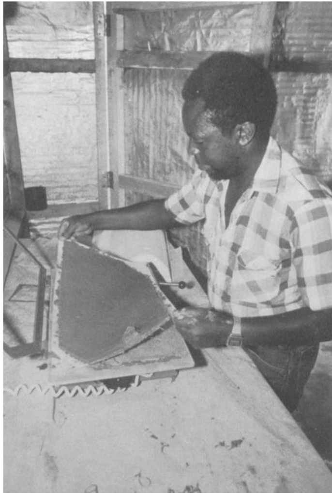
Figure 8.1 Manual fibre-concrete tile-making using the Parry process (from ITDG).
