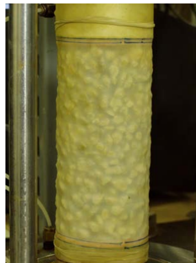
Fig. 1.29 Appearance of Chiba gravel specimen undergoing 1 kPa of effective stress
