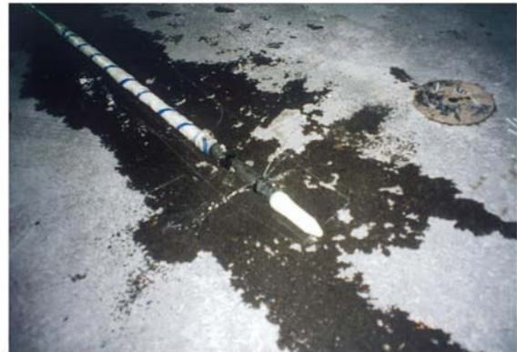
Fig. 26.120 Example of nozzle for injection of liquid (Pentaocean Inc.)
