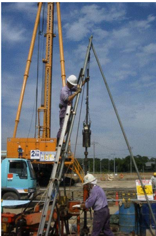
Fig. 1.38 Example of free-fall standard penetration equipment
