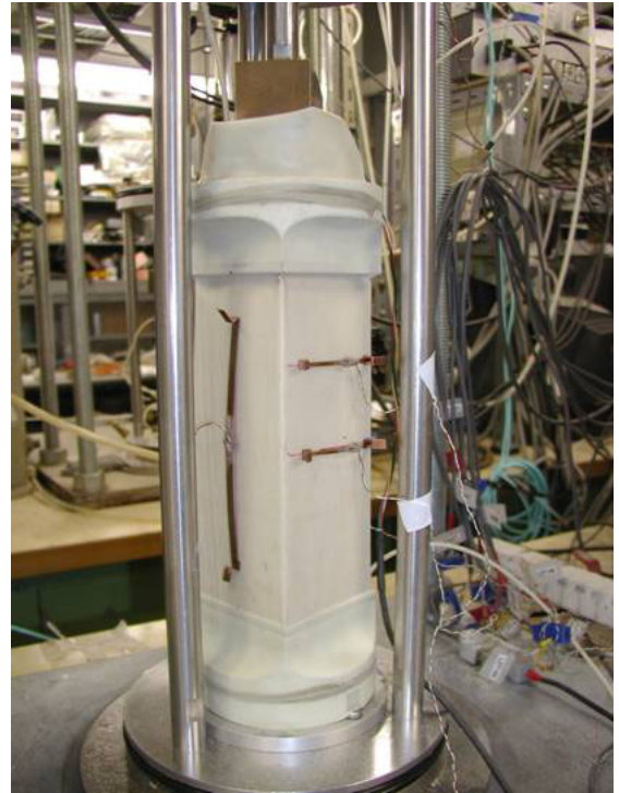
Fig. 10.3 Local displacement transducer attached on triaxial shear specimen
