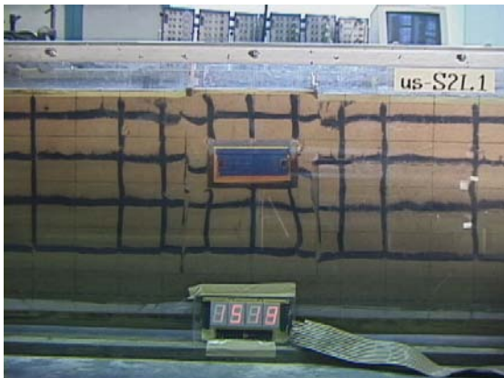
Fig. 24.51 Mitigation of liquefaction-induced floating of underground structure by installing sheet pile walls
