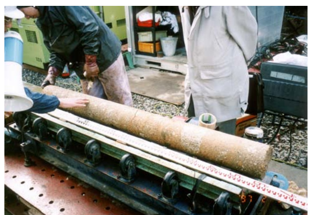
Fig. 10.64 Gravel particles at the surface of collected frozen specimen
