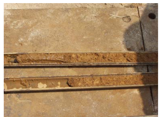
Fig. 1.37 Disturbed soil sample collected by tube
