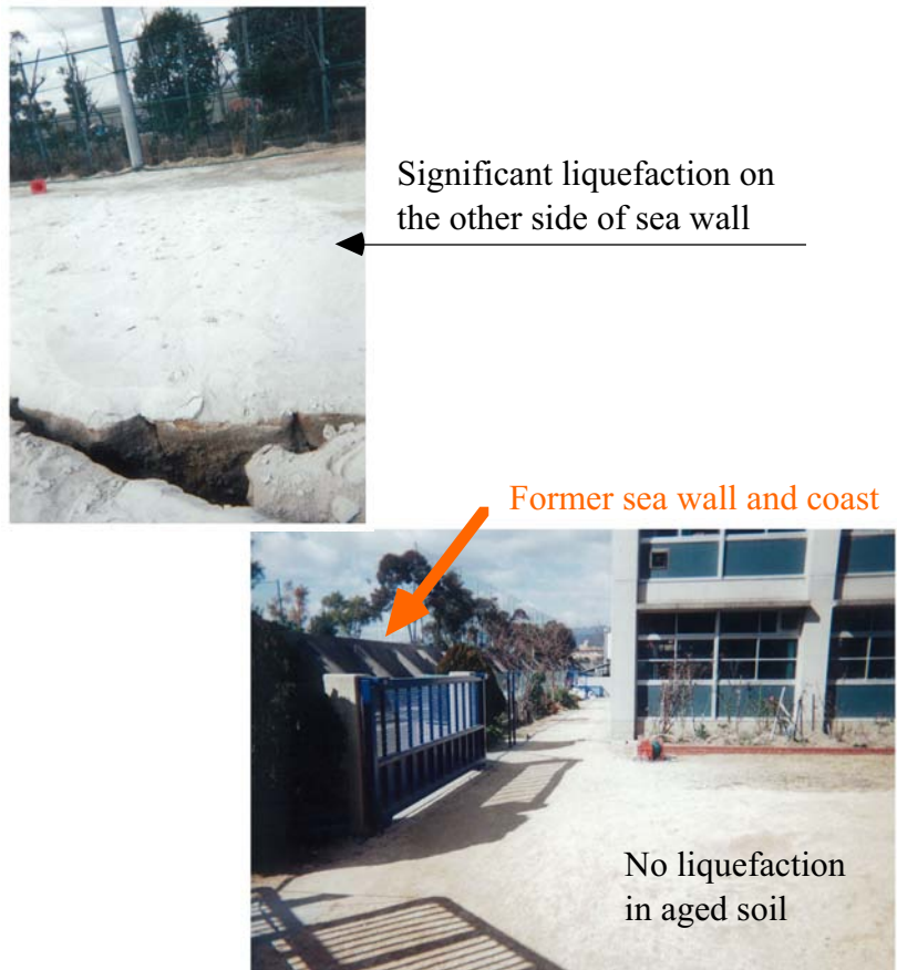
Fig. 18.45 Contrast in liquefaction resistance due to age difference
