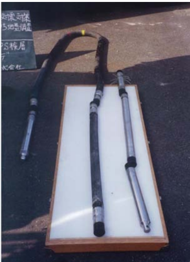
Fig. 8.6 Suspension survey equipment on site
