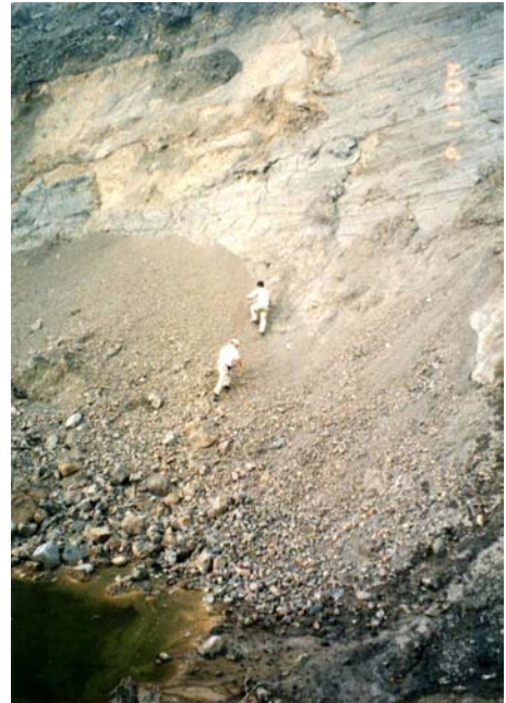
Fig. 15.2 Exposed slip plane in Galdian landslide
