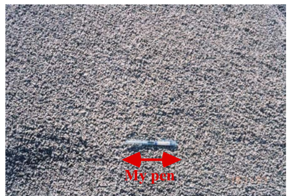
Fig. 26.87 Gravel particles employed for drain (see a ball point pen on gravel)
