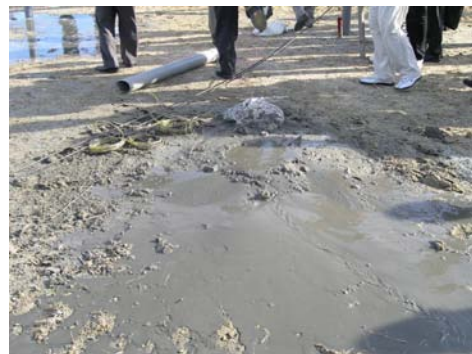
Fig. 26.142 Liquefaction caused by blasting
