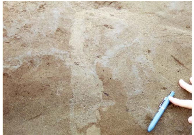
Fig. 18.13 Channel of boiled sand (Sekiyado)
