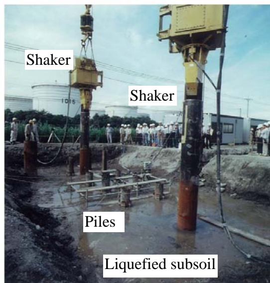
Fig. 26.93 Field liquefaction test on lateral rigidity of piles (Sumitomo Metal Industries)
