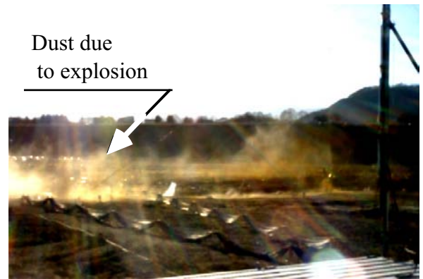
Fig. 18.14 Explosion to trigger liquefaction
