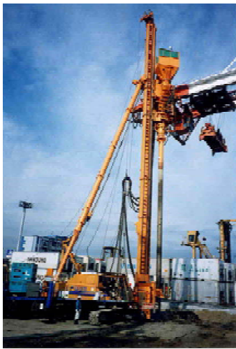
Fig. 26.62 Machine for silent construction of sand compaction piles
