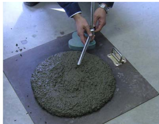
Fig. 26.140 Fluid nature of fluidized soil
