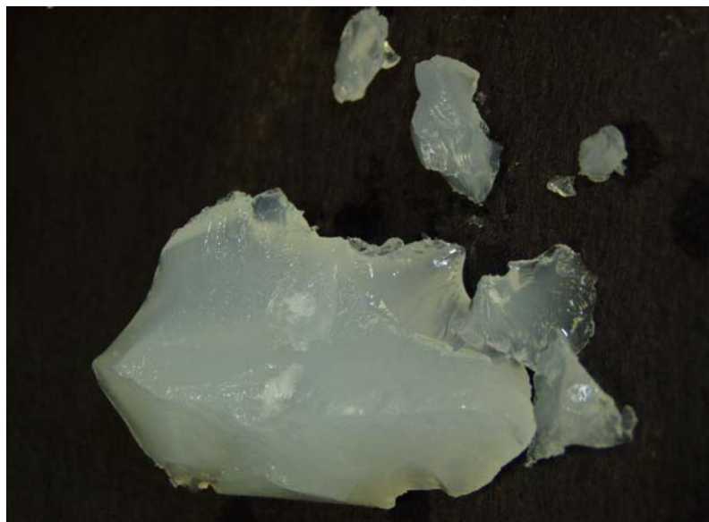
Fig. 26.132 Appearance of pure colloidal silica after curing
