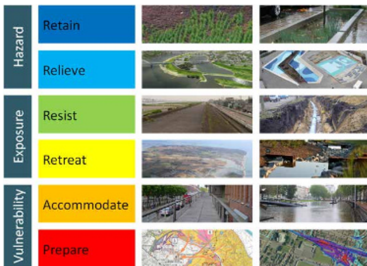
Figure 5-1 4-RAP model of available strategies – where the 4R's signify the retain, relieve, resist and retreat strategies; 'A' signifies accommodate strategy; and 'P' signifies prepare strategy - to enhance flood resilience (Adapted from Gersonius et al. (2016))
