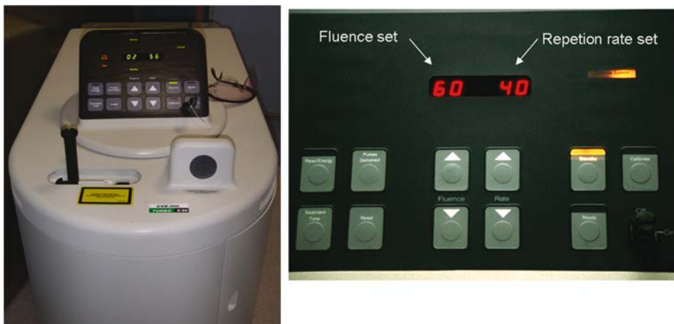
Figure 11.17 Panel a Spectranetics CVX-300 Excimer XeCl laser system. Panel b Laser consol. The arrows indicate fluence set and repetition rate set
