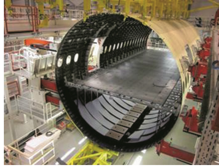
Fig. 2. Image of Airbus A350 XWB rear fuselage Section 16 at the assembly station
