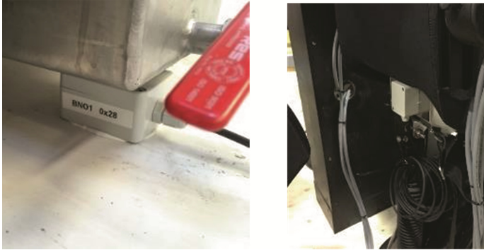
Fig. 3. Bosch BNO055 IMU sensor installations on Hydrolift P-42
