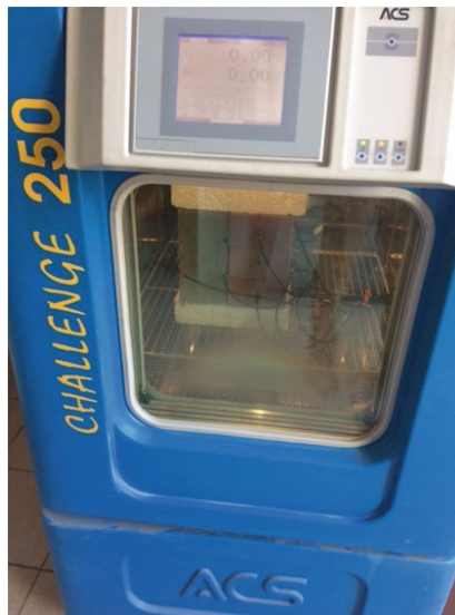
Fig. 1. Thermal Chamber used during the experiments
