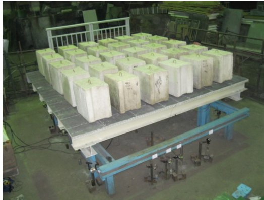
Fig. 4. The fragment before the test under load of 737 kgf/m 2 .
