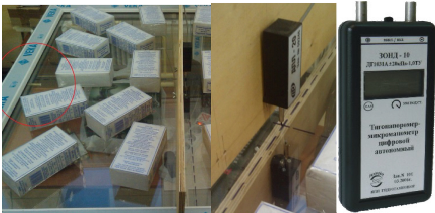
Fig. 5. (a) pneumatic valve for creating internal pressure in the pane; (b) measuring devices – digital deflection meters of linear type and digital micro pressure gage
