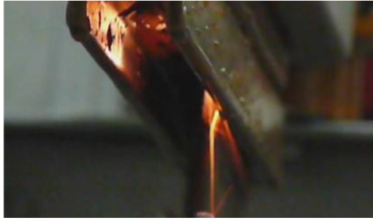
Fig. 6. Sparking in PMG-current distributor tribopair contact in increased humidity.
