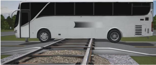
Fig. 7. Bus with large axle distance that was stuck at the level crossing in Biloxi, Mississippi on February 8 th 2017 [7].
