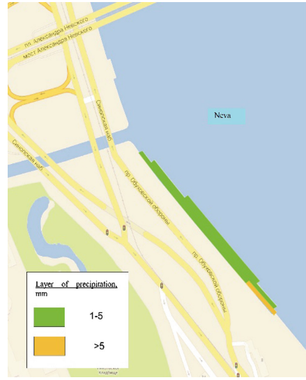
Fig. 4. Calculated field of thickness of the layer of suspended solids during the reconstruction of the Sinopskaya embankment.
