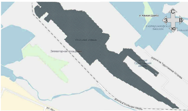
Fig. 6. Calculation grid for modeling the transport of suspended solids.
