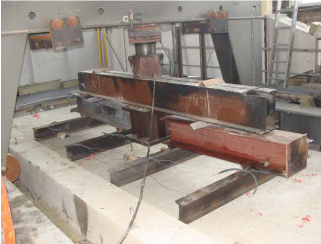
Fig. 2. An experimental sample of a reinforced concrete slab of a ceiling installed on the fire chamber of a test installation with an applied static load in accordance with the design scheme.
