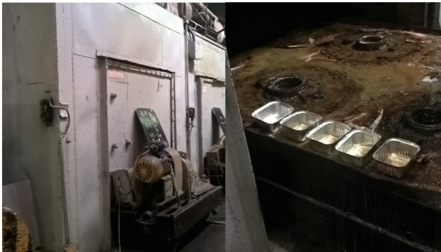
Fig. 7. Samples installation into the convection oven
