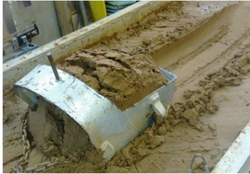
Fig. 3. Bucket-chain model at the end of an excavation run.
