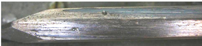
Fig. 8. Grooves from fine disperse particles on the copper graphite contact element.
