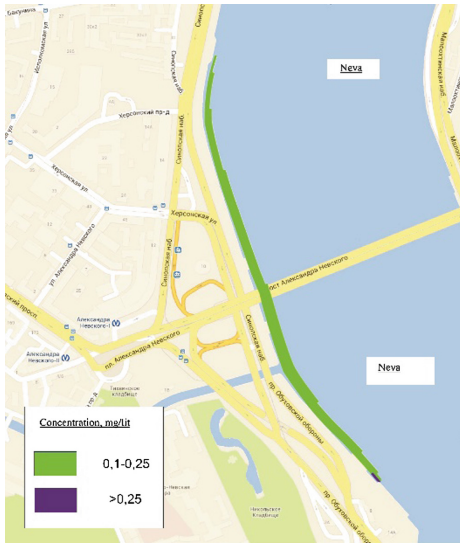
Fig. 3. Calculated field of concentrations (mg/lit) for the reconstruction of the Sinopskaya embankment.
