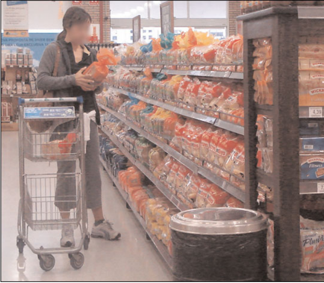
Figure 3.3 Sloping shelves create a sense of greater openness without expanding the aisle width at floor level.
