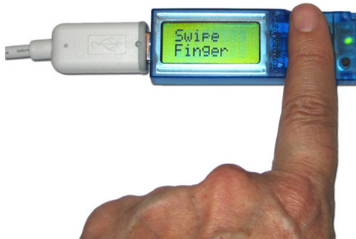
Figure 4. Fingerprint authentication technology allows customers to pay for purchases with only the press of a finger
