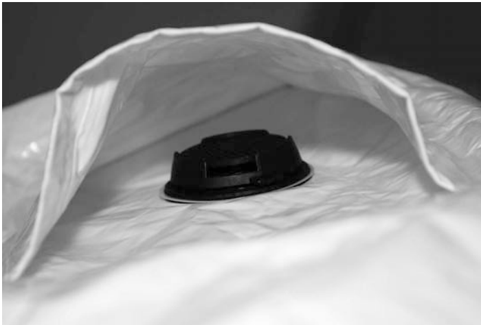
PHOTO 20.21 Outside of Level A vapor-proof suit: Both the outside protective “tent” made of impermeable suit material and the outside rigid housing of the one-way air valve (air flow direction from inside to outside of suit) are seen in this photograph. A flapper disc made of chemically impermeable material (often halogenated butyl rubber or EDPM rubber) is within this housing. (Author’s personal photos taken at Lakehurst, N.J. Naval Air Station. Thanks to Len Dotson, photographer and member of New Jersey Task Force 1 who spent a good deal of time serving as photographer and photographic advisor, and Sergeant Daniel Mitten of New Jersey Task Force 1 of the New Jersey State Police.)
