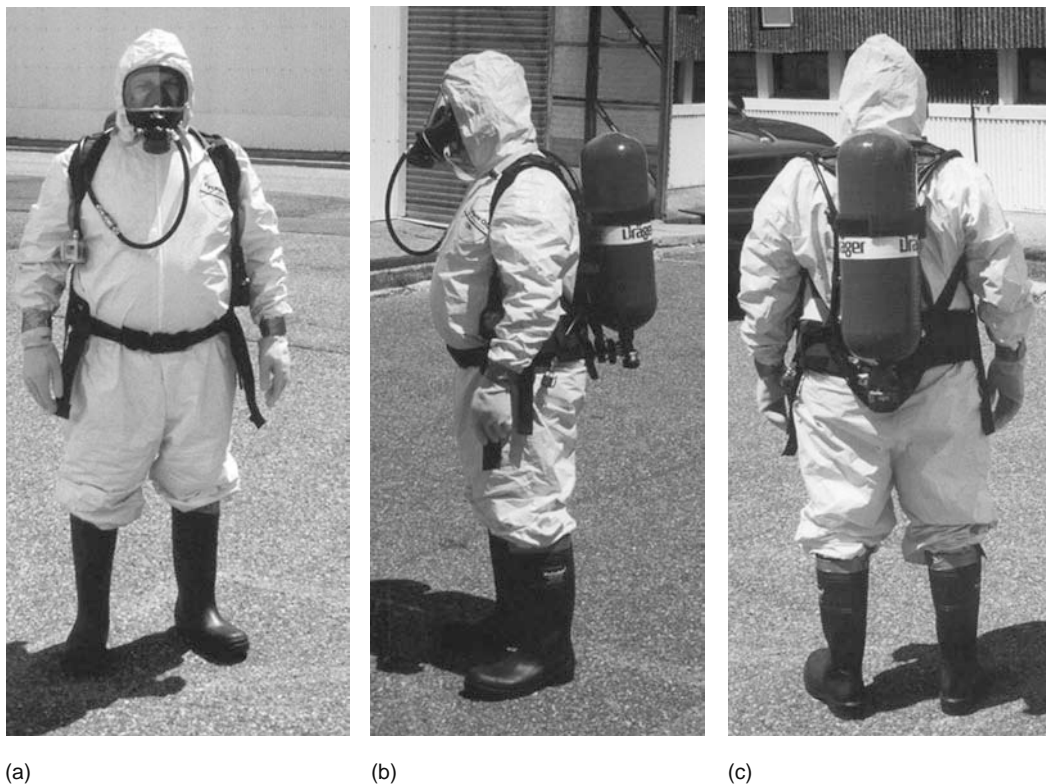
PHOTO 20.3 (a and b) Level B: Notice the taping of the gloves and boots to the outside of the suit. In addition note how some of the impermeable suit material overhangs the boots and is taped to the boots using duct tape (tape with known chemical agent permeation data would be preferable) with a “tear off” tab. Several layers of gloves are usually employed. (Author’s personal photos with him serving as the responder, taken at Lakehurst, N.J. Naval Air Station by Sergeant Daniel Mitten of New Jersey Task Force 1 and the New Jersey State Police.) (c) Level B: Another picture illustrating the support mechanism of the SCBA allowing it to ride on the hips. Notice how the tank is mounted with a tank shut-off valve and the first stage of the regulator (high-pressure reducing stage) is mounted under the tank. (Author’s personal photos with him serving as the responder, taken at Lakehurst, N.J. Naval Air Station by Sergeant Daniel Mitten of New Jersey Task Force 1 of the New Jersey State Police.)
