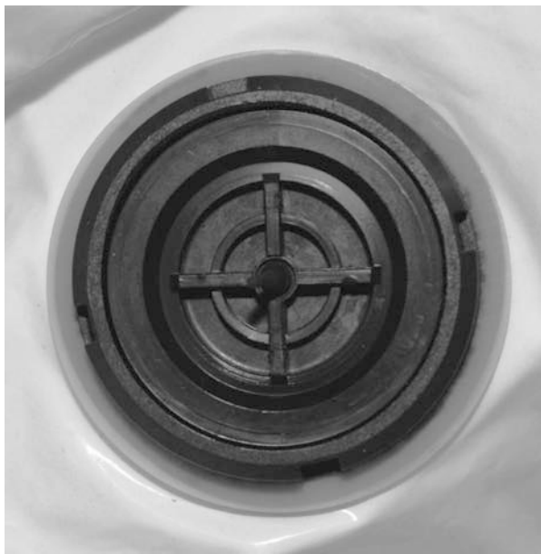
PHOTO 20.22 Inside of Level A vapor-proof suit: One can see the one-way air escape valve flapper disc that opens to the outside atmosphere when pressure within the suit exceeds atmospheric pressure. As soon as the pressure is equalized the disc valve closes. Sticking of this air escape valves mechanism would cause air expired from the SCBA to be retained within the suit and increase pressure within the suit, buildup of pressure could rupture the suit. One should always be sure these valves are functioning properly before donning the suit. (Author’s personal photos taken at Lakehurst, N.J. Naval Air Station. Thanks to Len Dotson, photographer and member of New Jersey Task Force 1 who spent a good deal of time serving as photographer and photographic advisor, and Sergeant Daniel Mitten of New Jersey Task Force 1 of the New Jersey State Police.)
